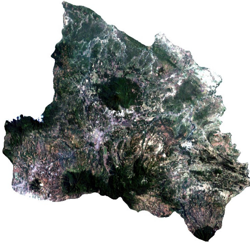
Fig 4. Composite Band of Landsat 7 Image in 2013. Band combination (3-2-1) were applied to create the composite image where band 3 is Red, band 2 is Green, and band 1 is Blue. This satellite image captures the land cover and vegetation patterns in 2013.
