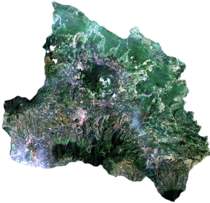
Fig 3. Composite Band of Landsat 7 Satellite Image in 2003. Band combination (3-2-1) were applied to create the composite image where band 3 is Red, band 2 is Green, and band 1 is Blue. This satellite image captures the land cover and vegetation patterns in 2003.
