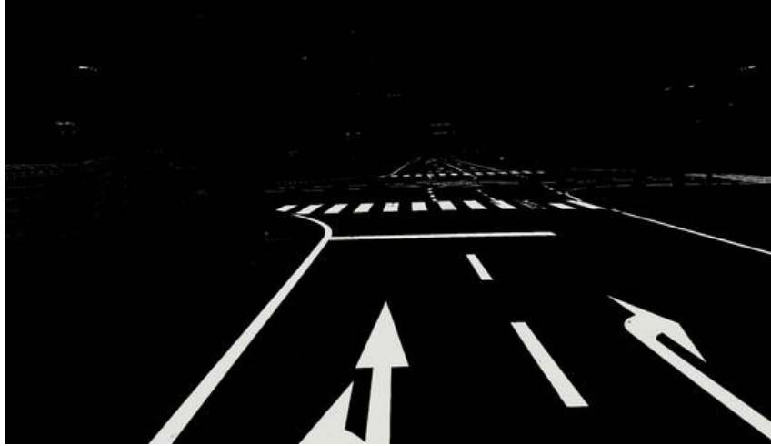
Figure 3.4: Output of K-means and Pixels Selection of Cluster with Highest Mean
