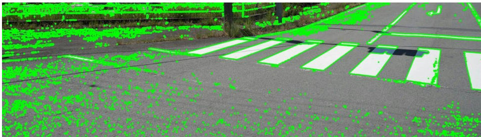
Figure 3.9: Applying the Jarvis algorithm outputs' contours which are sets of pixels delimiting a certain cluster of pixels in the image, for each contour we will compute the "Smoothness".
