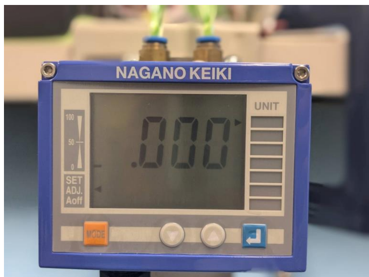
Figure 3.14. GC 50 multifunctional digital differential pressure gauge.
