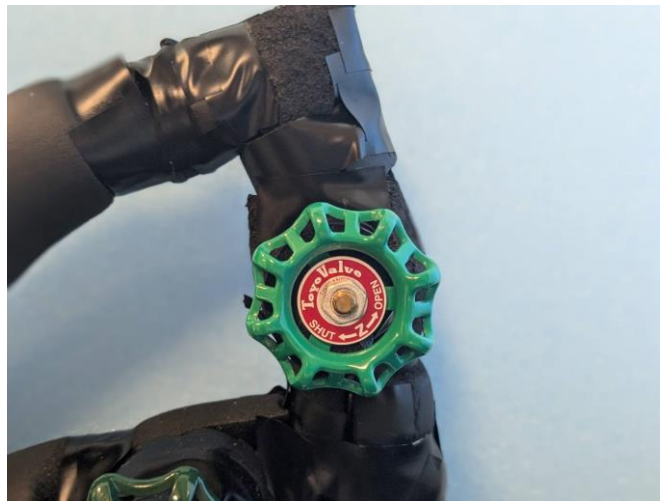
Figure 3.16. Globe valve for controlling flow rate.
