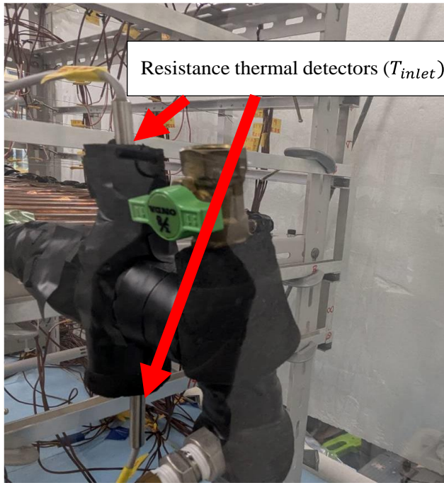
(b) Physical photo of inlet fluid temperature measurement
