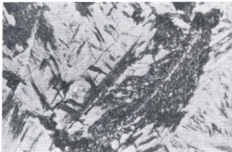
S45C preheating temp. 100°C bainite martensite
