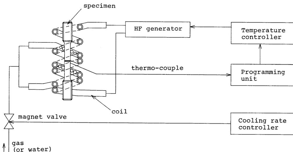
Fig.1 Simulator of weld-thermal-cycle
