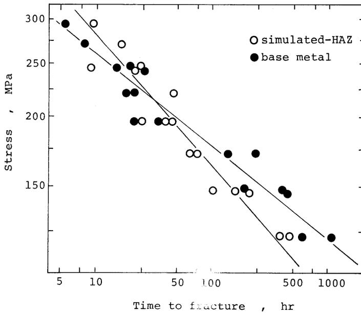
Fig. 6 Results of creep-rupture test on simulated-HAZ and base metal of 1 1/4Cr-1/2Mo steel
