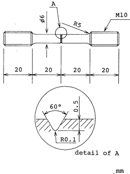
Fig. 5 Specimen for creep-rupture test
