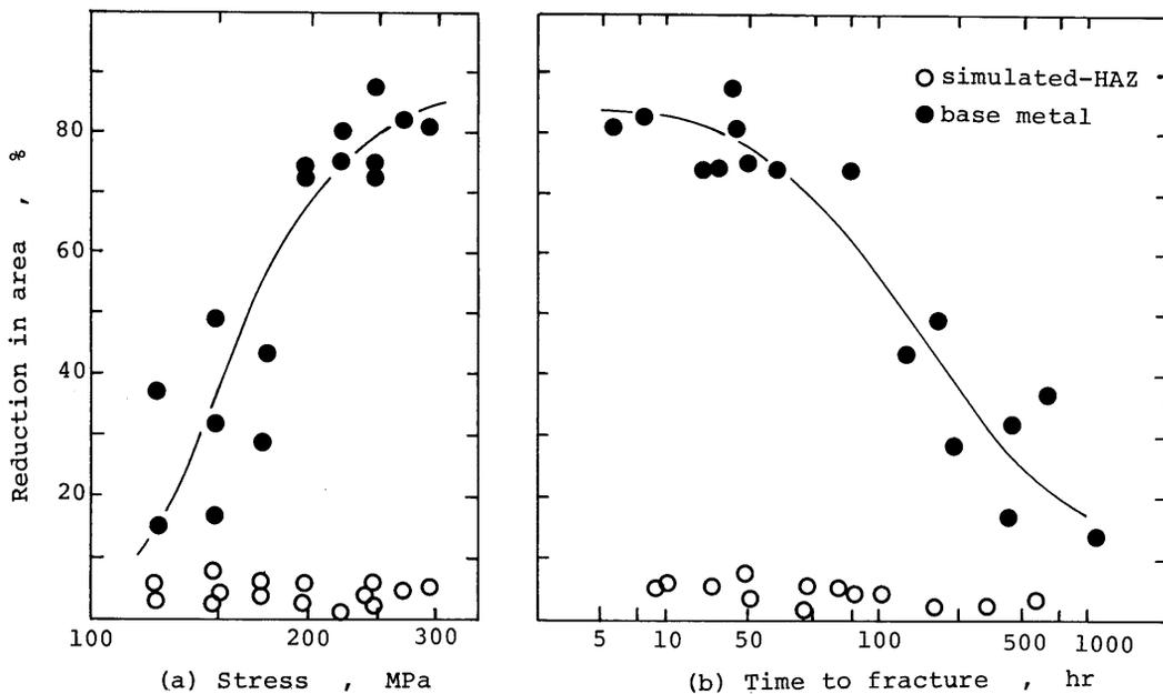
Fig.7 Reduction in area shown by the parameters of stress (a) and time to fracture (b)
