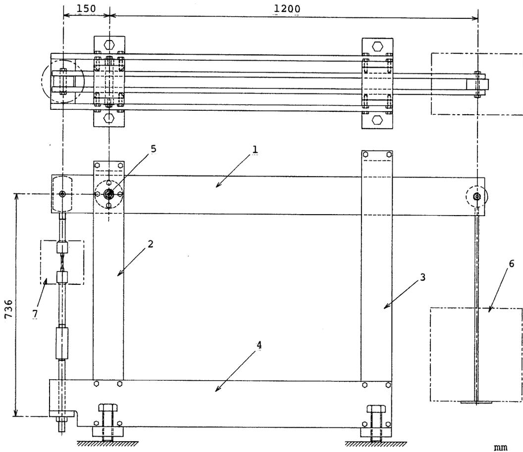
Fig.3 Creep-test machine for LDCF and TEIC
