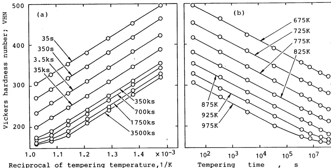
Fig.4 Influences of temperature (a) and time (b) on the tempered hardness of S55C steel
