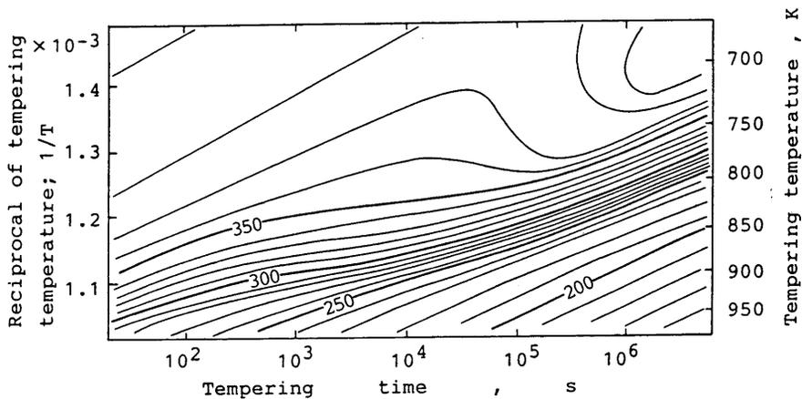
Fig. 15 The time-temperature-hardness diagram of 2 1/4Cr-1Mo steel
