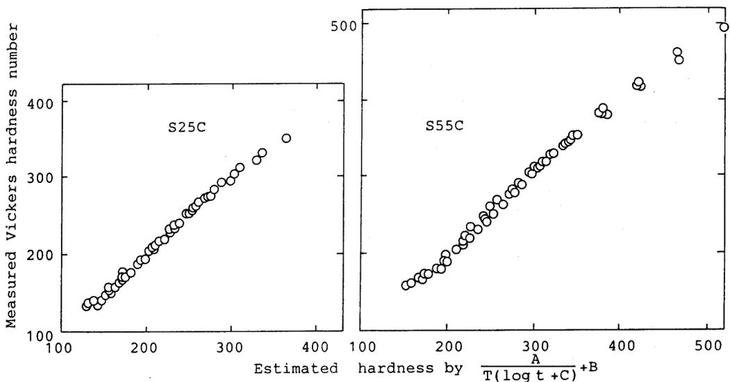
Fig.7 The tempered hardness of S25C and S55C steels comparing with the estimated value by eq.(8)
