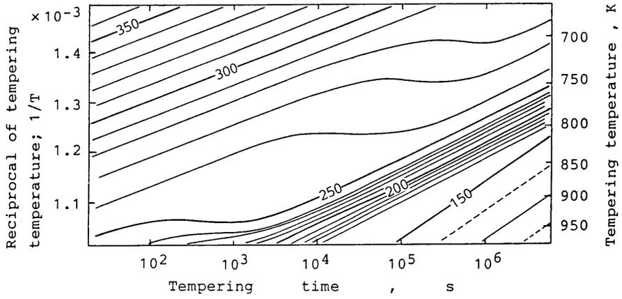
Fig.11 The time-temperature-hardness diagram of HT60 steel
