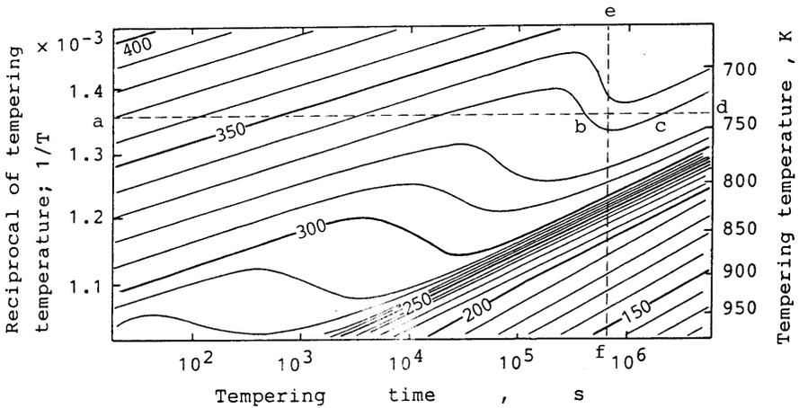
Fig.13 The time-temperature-hardness diagram of 1/2Mo steel
