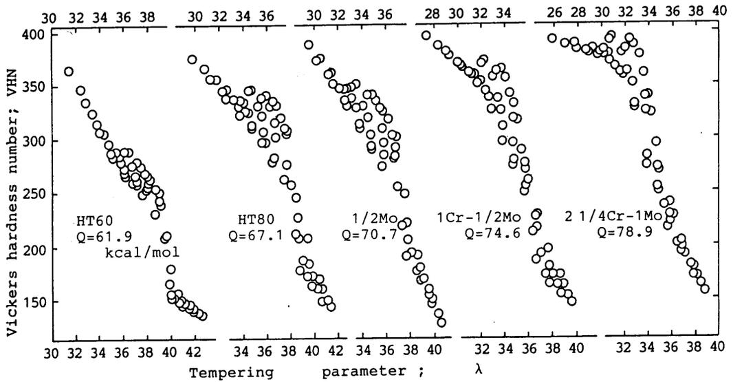
Fig.9 The tempered hardness of HT60, HT80, 1/2Mo, 1Cr-1/2Mo and 2 1/4Cr-1Mo steels against the parameter,  $\lambda$
