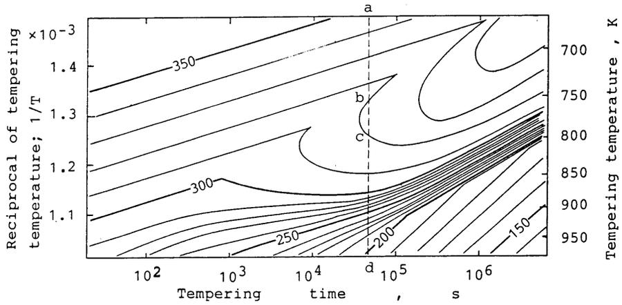
Fig.12 The-time-temperature-hardness diagram of HT80 steel
