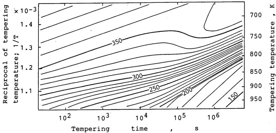
Fig. 14 The time-temperature-hardness diagram of 1Cr-1/2Mo steel
