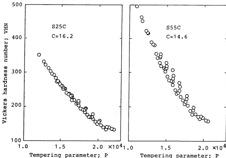
Fig.6 The tempered hardness of S25C and S55C steels against the parameter, P
