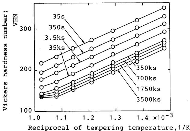
Fig.3 The tempered hardness of S25C steel against the reciprocal of tempering temperature, 1/T
