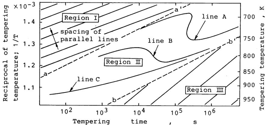
Fig.10 Schematic illustration of the time-temperature-hardness diagram
