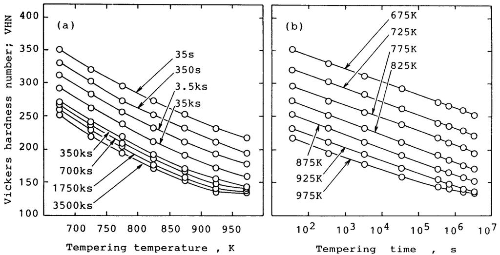
Fig.2 Influences of temperature (a) and time (b) on the tempered hardness of S25C steel
