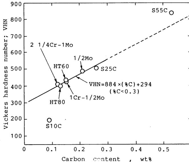
Fig.1 As-quenched hardness of steels against the carbon content
