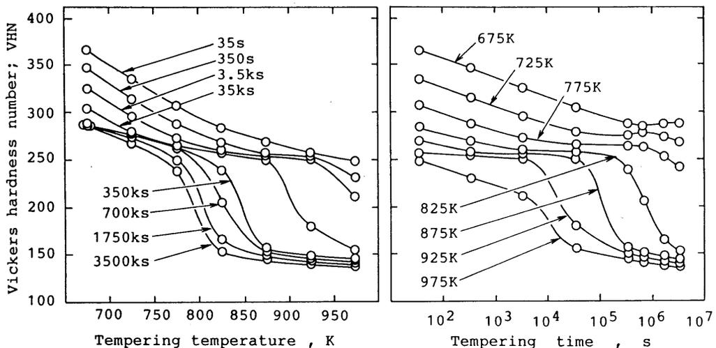
Fig.8 Influences of temperature and time on the tempered hardness of HT60 steel
