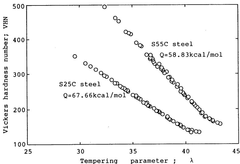
Fig.5 The tempered hardness of S25C and S55C steels against the parameter, λ
