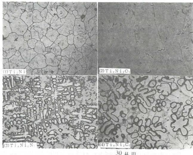
Fig.3 Crystal Structures of  $Ti_4Ni_2X$  Intermetallic compounds
