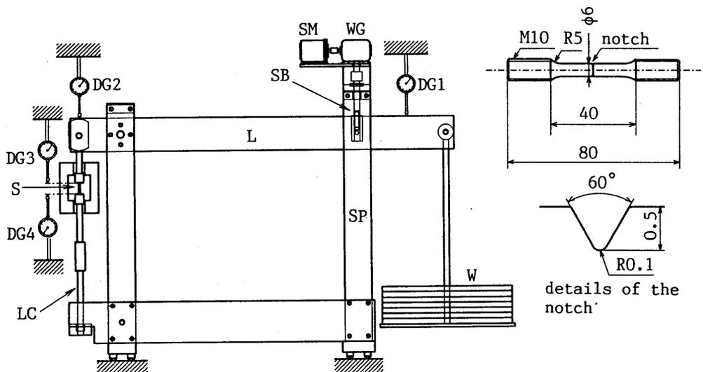
Fig.1 The apparatus for the cracking test and the dimensions of the specimen
