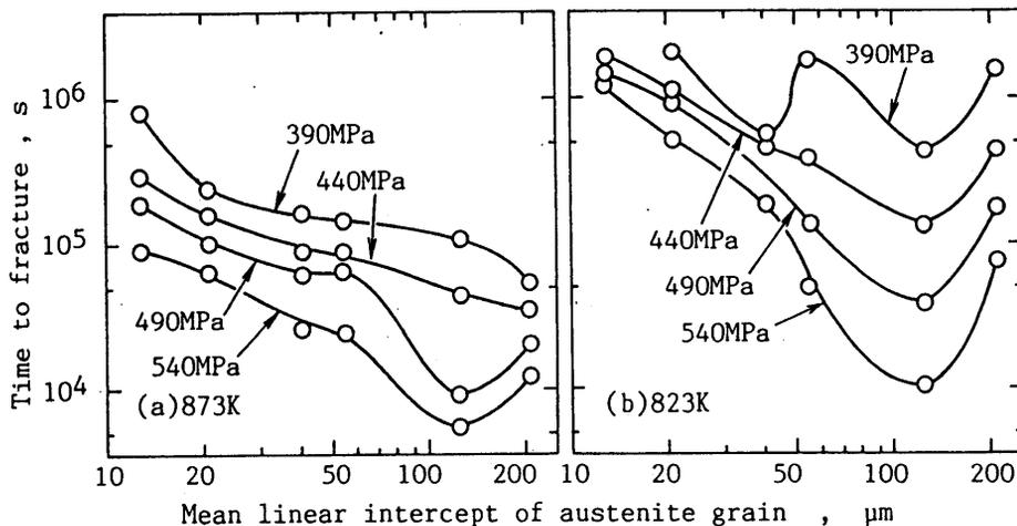
Fig.5 The effect of grain size on the time to fracture for the constant load test
