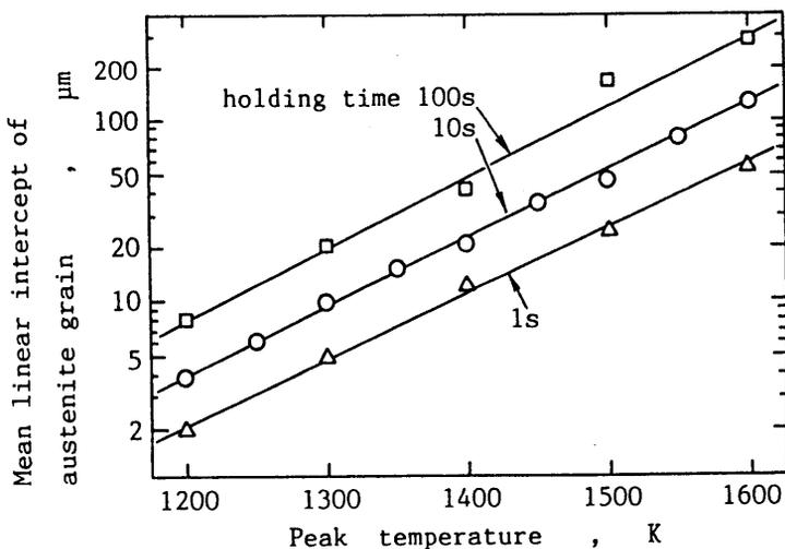
Fig.3 The effect of processing parameters on the size of austenite grain
