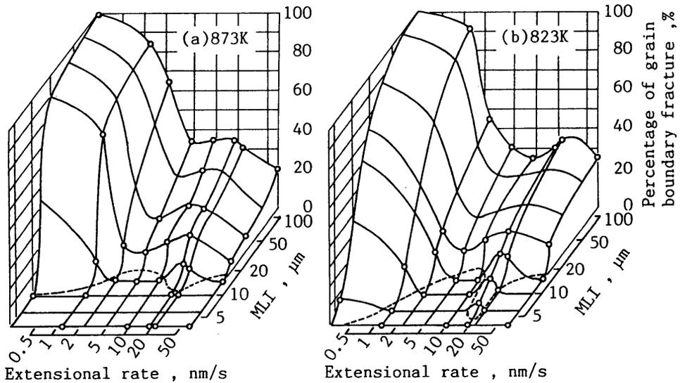
Fig.7 The percentage of grain boundary fracture for the constant extensional rate test
