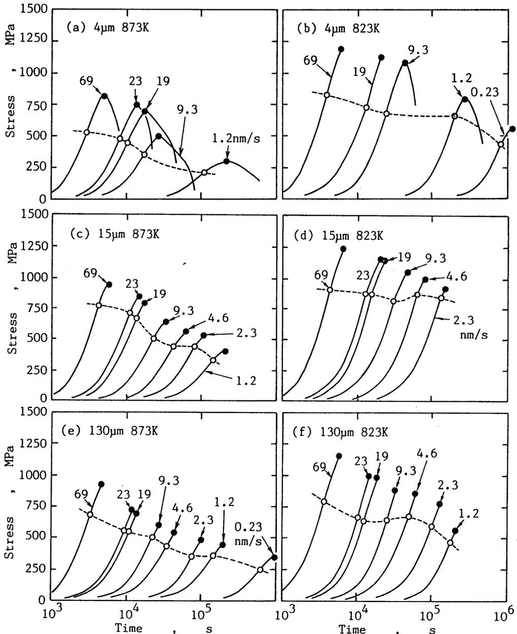
Fig.6 The stress curves obtained by the constant extensional rate test
