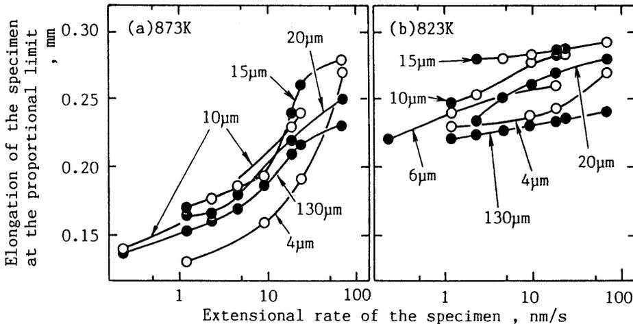
Fig.11 The elongation of the specimen at the proportional limit of the stress curve
