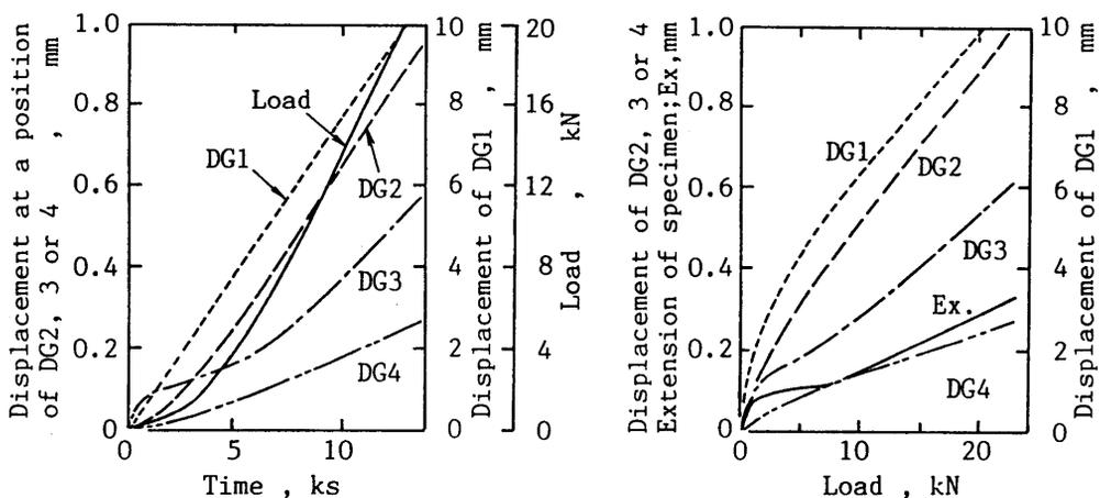
Fig.2 The elastic deformations of the testing machine under loading
