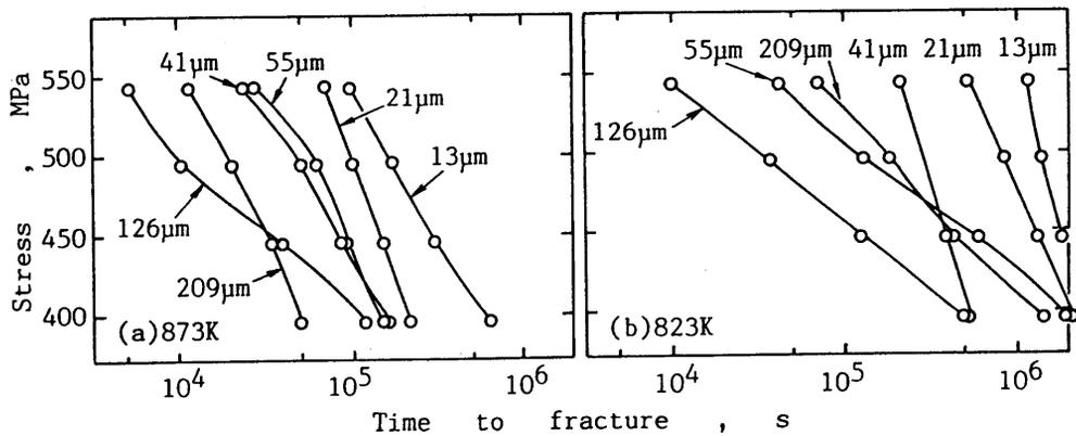
Fig.4 The time to fracture obtained by the constant load test
