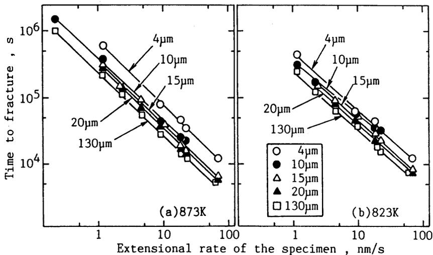
Fig.9 The relation between the extensional rate and the time to fracture
