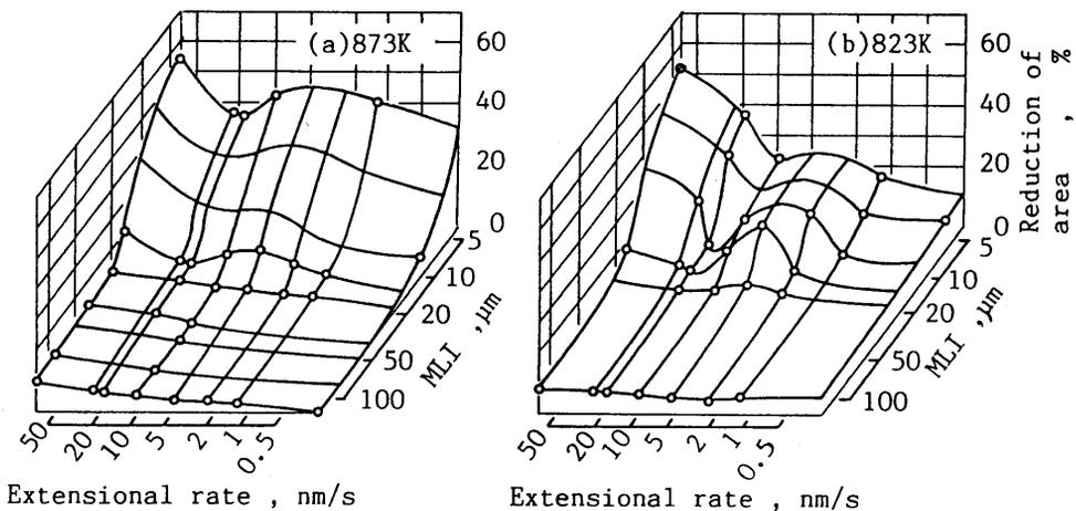
Fig.8 The reduction of area for the constant extensional rate test
