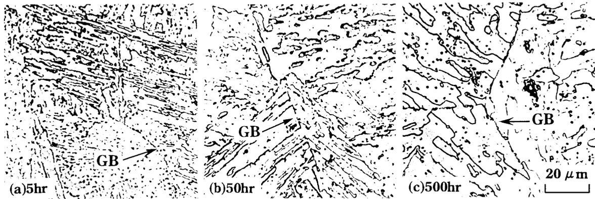
Fig.11 Change of morphology of ferrite grains with an increasing tempering time at 975K; GB: grain boundary of prior-austenite.
