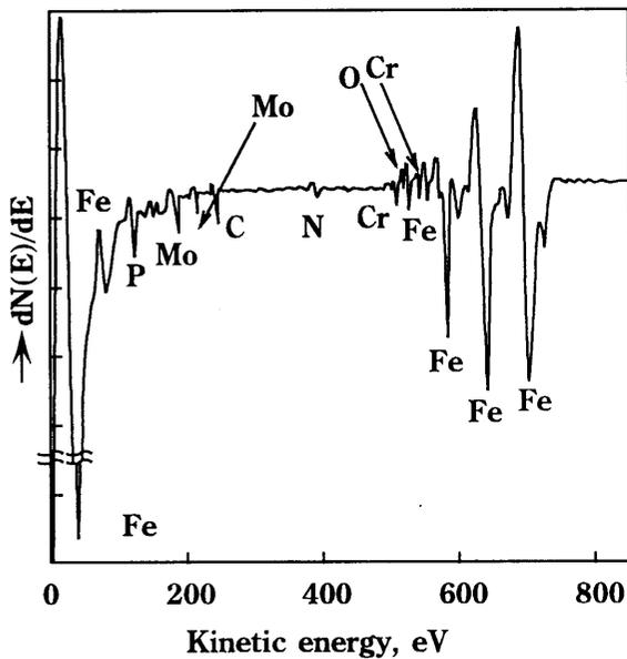
Fig.14 Auger spectra showing the segregation of impurities at grain boundary; specimen was suffered from the third type of embrittlement.
