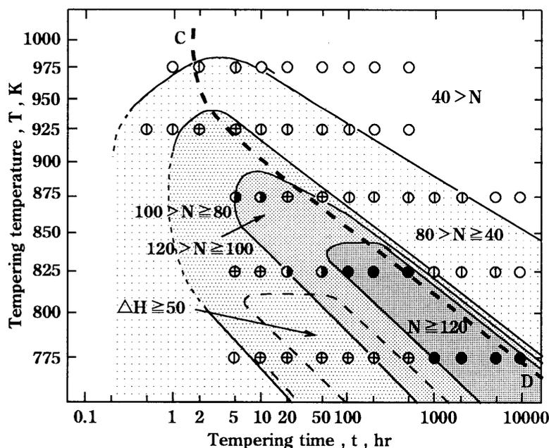
Fig.7 Numbers of carbide particles in  $5 \mu m$  square,  $N$  shown in the tempering temperature-time diagram; CD line: beginning of the growth of carbide particles; ●  $N \geq 120$ , ○  $120 > N \geq 100$ , ⊕  $100 > N \geq 80$ , ⊖  $80 > N \geq 40$ , ○  $40 > N$ .
