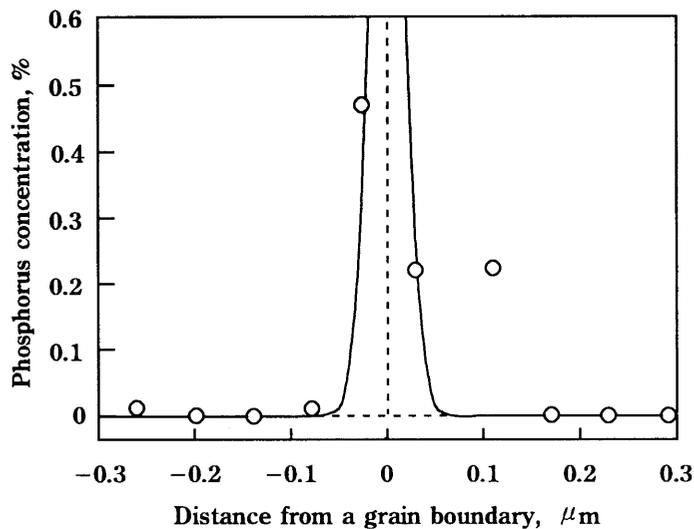
Fig.15 Phosphorus concentration in the grain boundary measured by point counting method in EDX analysis; specimens was suffered from the third type of embrittlement.
