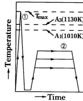
Fig.2 Thermal cycles given to HAZ during and after welding, ①Welding, ②Tempering,
