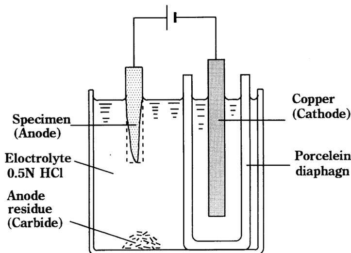
**Fig.9 Apparatus for electrolytic extraction of carbide.**
