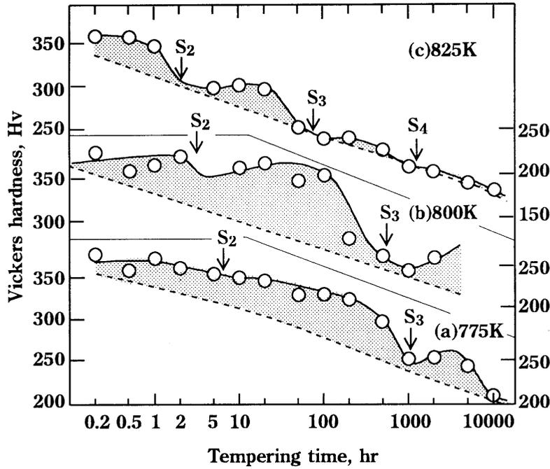
Fig.5 Change of hardness with the lapse of tempering time at 775K to 825K.
