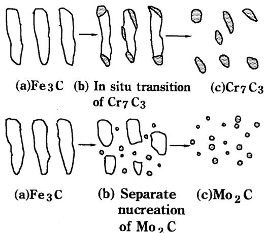
Fig.4 Different nucleation systems of  $Cr_7C_3$  and  $Mo_2C$ .
