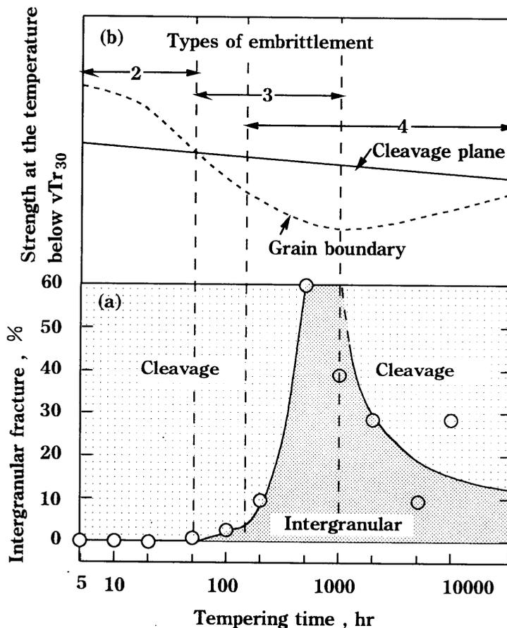
Fig.13 Intergranular fracture brought about by the decrease of grain boundary strength in the time range where the third type of embrittlement arises.
