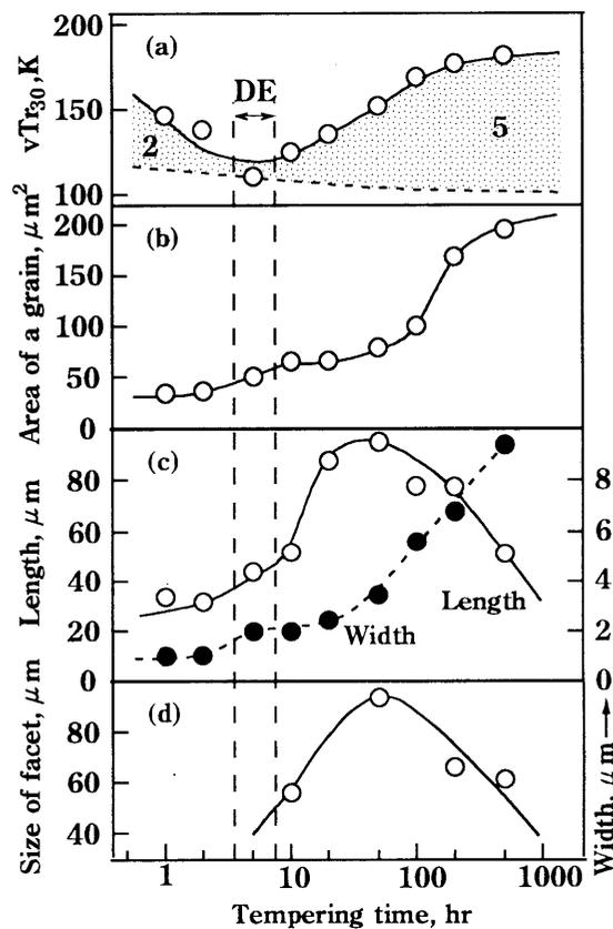
Fig.12 Change in size and shape of ferrite grains with an increasing tempering time at 975K and their effects on the fifth type of temper embrittlement.
