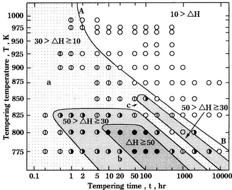
Fig.6 Increment of hardness  $\Delta H$  induced by secondary hardening shown in tempering temperature–time diagram;
