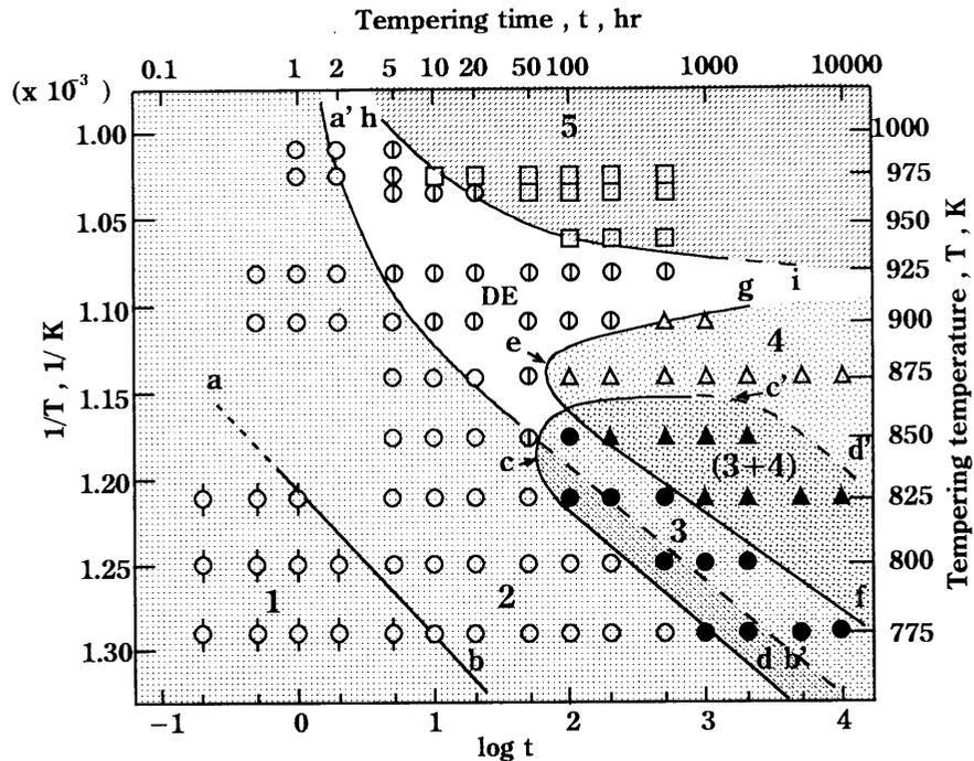
Fig.3 Tempering temperature–time fields where five types of temper embrittlement arise in 2 1/4Cr–1Mo steel; Marks show the specimen in the embrittled state of;  $\circ$  first type,  $\square$  second type,  $\bullet$  third type,  $\Delta$  fourth type,  $\blacktriangle$  third and fourth type,  $\square$  fifth type,  $\oplus$  de-embrittle state.
