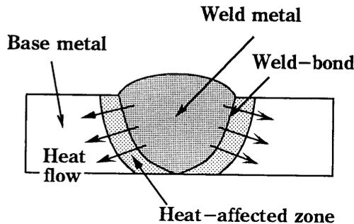
Fig.1 Welded zone produced by arc welding.
