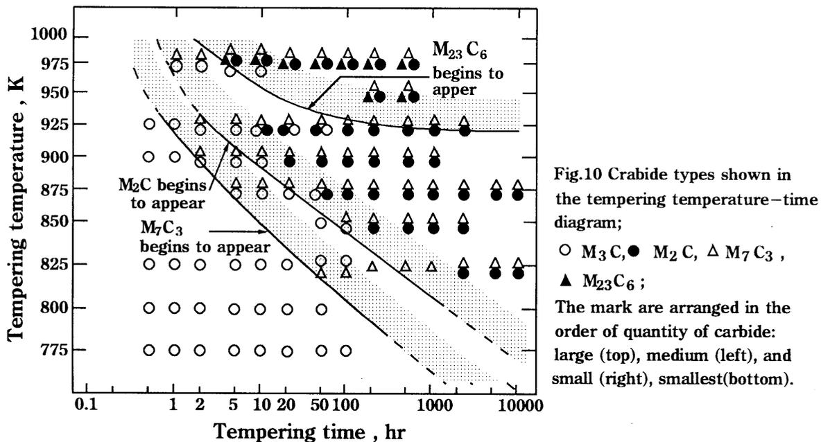
Fig.10 Carbide types shown in the tempering temperature-time diagram;
