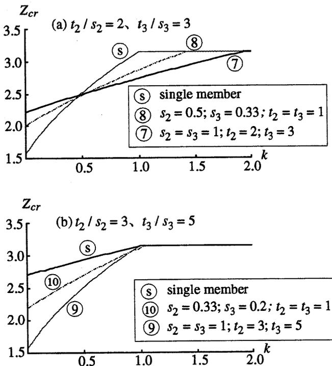
Fig. 14 Comparison of  $Z_{cr} - k$  Curves:  $t_i/s_i = \text{const.}$  ( $n = 3$ )
