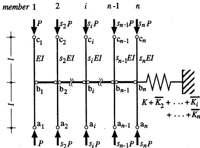
Fig. 7 Replaced Model with Additional Springs
