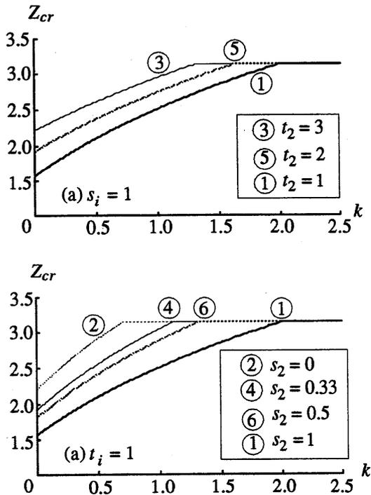
Fig. 12 Effects of Load Ratio and Stiffness Ratio ( $n = 2$ )
