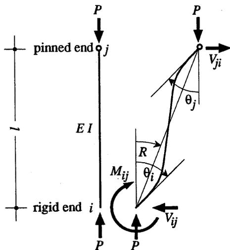
Fig. 1 Deformed Member Subjected to End Forces
