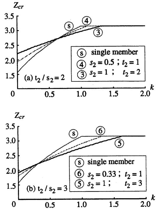
Fig. 13 Comparison of  $Z_{cr} - k$  Curves  $t_i/s_i = \text{const.}$  ( $n = 2$ )
