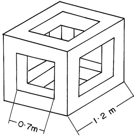
Fig. 4. A sketch of a concrete shelter. It weighs ca. 1.5 tons.
