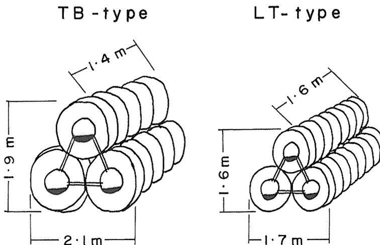
**Fig. 6.** Sketches of two types of unit tier shelters. TB-type shelter weighs ca. 1.7 tons, LT-type shelter weighs ca. 1.4 tons.
