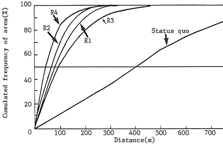
Figure 23. Scatter diagram of *area increase of service zone* within the alternative route; the *geometric off-road transport distance*.
