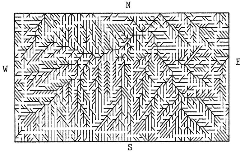
Figure 8. Network of stream lines derived from DTM's slope elements.
