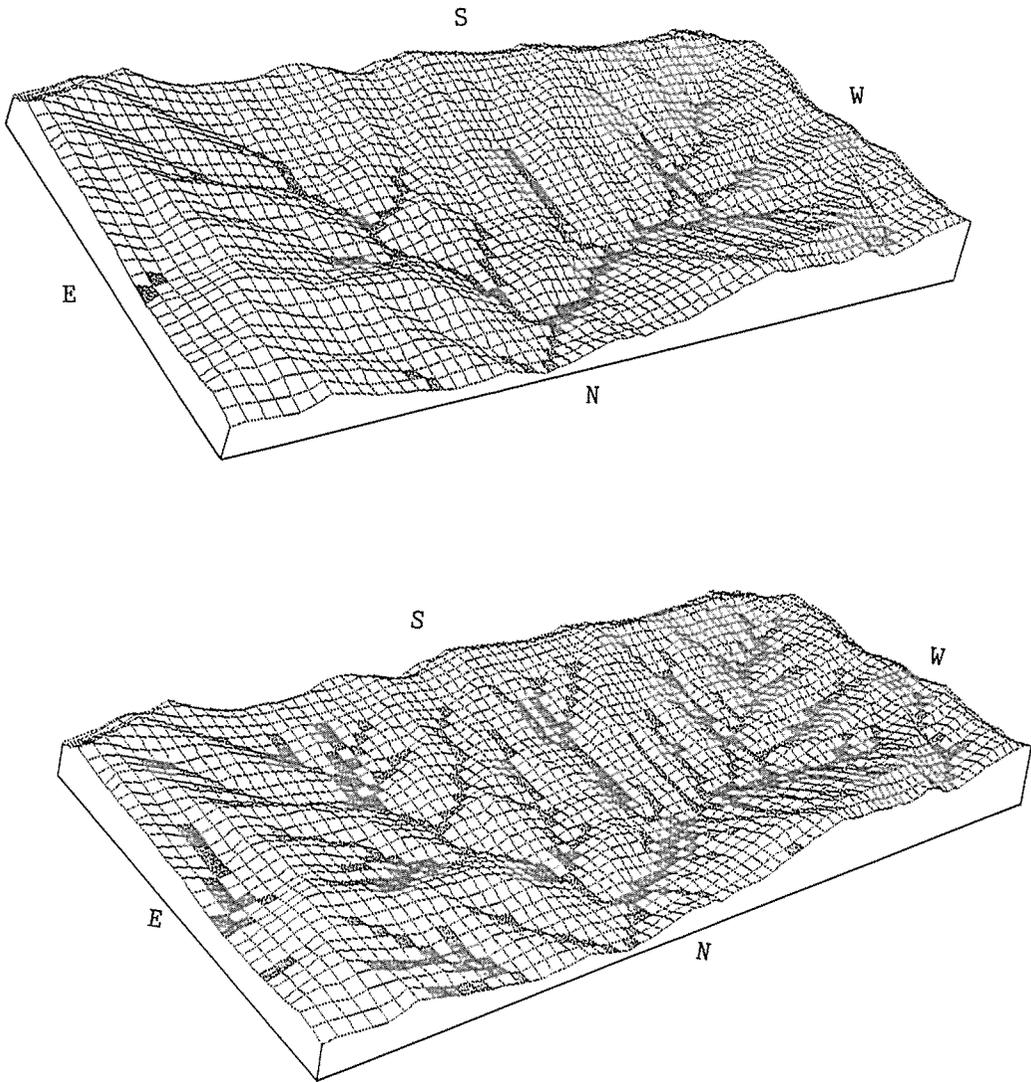
Figure 10. Comparison of two drainage patterns set at 5 ha (upper) and 1 ha (lower) drainage area.
