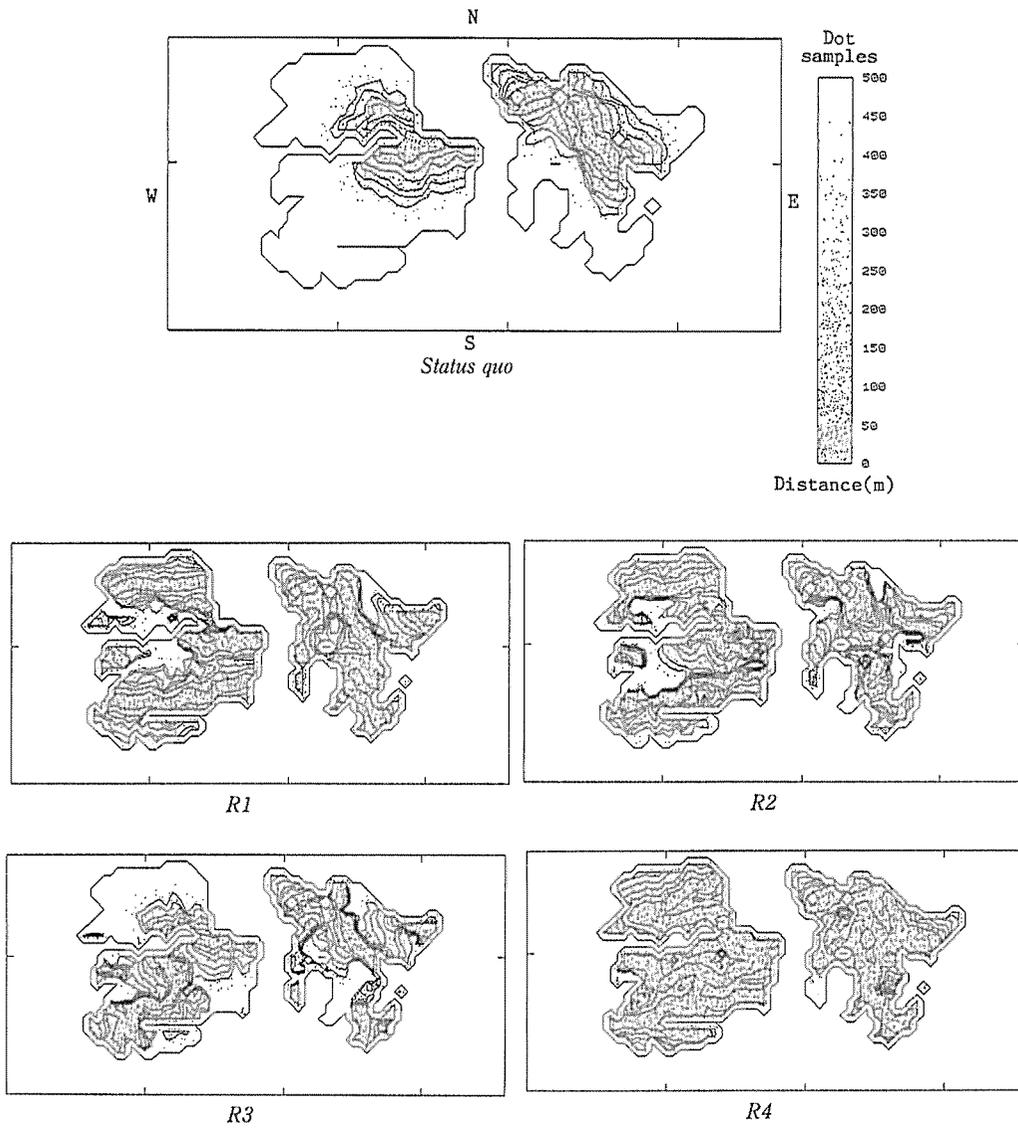
Figure 22. Voronoi map showing the service zone within the alternative route; the actual off-road transport distance. Contour interval is 50 m and dot samples also represent 50 m unit.
