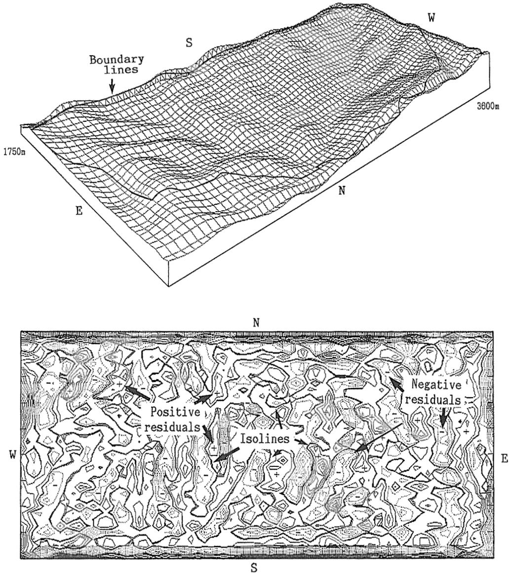
**Figure 11.** The configuration of the *Fourier trend surface model* obtained by applying the double Fourier series to the DTM surface (upper), using *MAICE* theory (*Minimum AIC Estimation*) which is statistic estimates of the Kullback-Leibler information criterion, and the *residuals* which are the remainder found by subtracting the actual from the computed trend surface value (lower); contour interval of residuals is set at 10 m.
