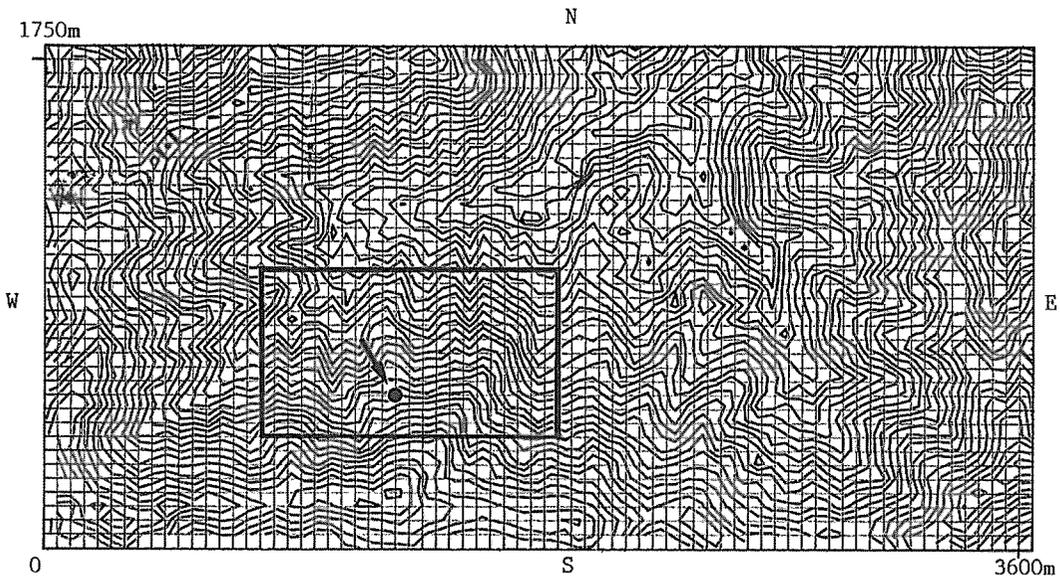
**Figure 3b.** Computer-generated digital contour map (contour interval: 20 m) with the square grid of the DTM (50 m×50 m); Rectangular portion of the grid blocks bounded by bold lines indicates the model area designed for visual landscape modification by generating perspective drawings shown in **Figure 17** and also the arrowhead shows the specific grid-intersection used to solve for viewing range of the terrain from the selected viewpoint in the DTM coverage area in **Figure 16**.
