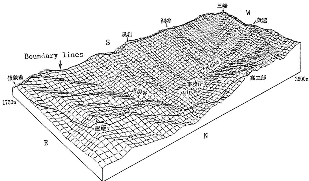
Figure 4. Perspective plot of the DTM surface in the study site; gridline spacing is set at 50 m. Arrowheads indicate the dominant drainage basins and ridges. Bold line shows boundary of the Mie University Forest.
