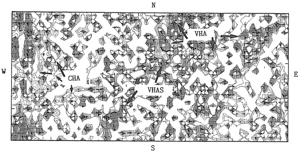
Figure 7. Delineation of the appropriate boundaries of *terrain-harvesting system area*; dotted contour line is set at slope gradient of 10%.
