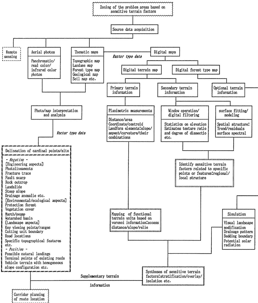
Figure 2. Functional components of the TERDAS, modules to suit various applications in opening-up planning process, such as route location or harvest system plan are added as required to this system.
