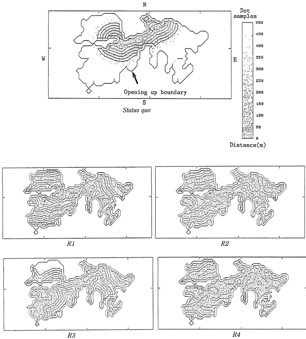
Figure 21. Voronoi map showing the service zone within the alternative route; the geometric off-road transport distance. Contour interval is 50 m and dot samples also represent 50 m unit.
