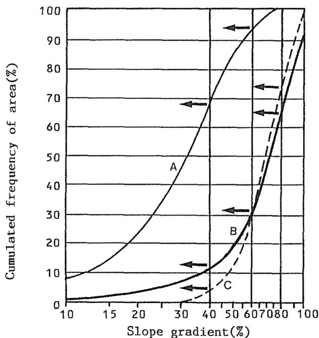
Figure 18. Terrain conditions of mountain forests associated with slope steepness (*cumulated slope frequency curve*); average slope gradient value is obtained by a resolution of all DTM grid cells per slope attribute cells.
