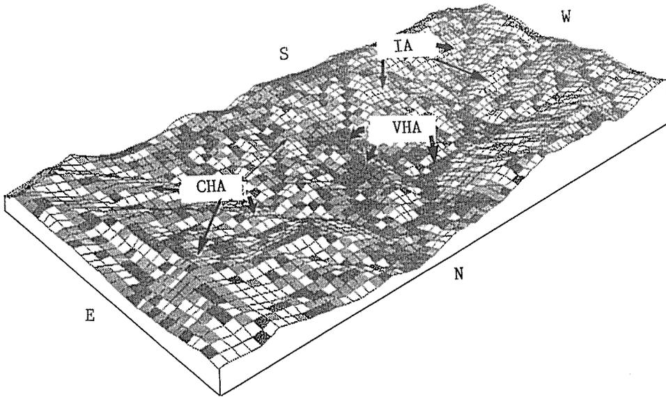
Figure 6. Subdivision of *terrain-harvesting system area* based on slope steepness; slope ranges as follows.
