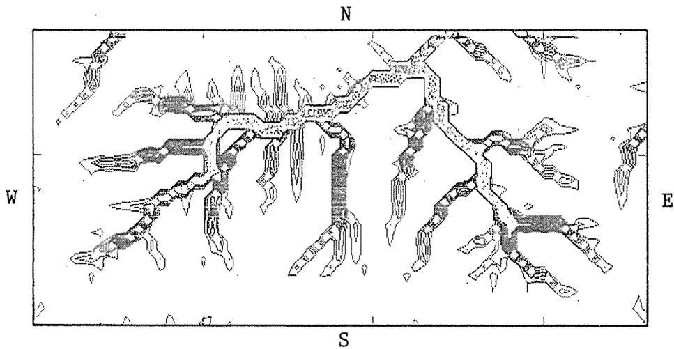
Figure 9. Delineation of the *drainage boundaries* by an interpolation algorithm; contour interval is set at drainage area of 1 ha.
