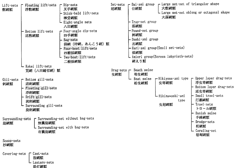
Fig. 1. Classification of netting gear.
