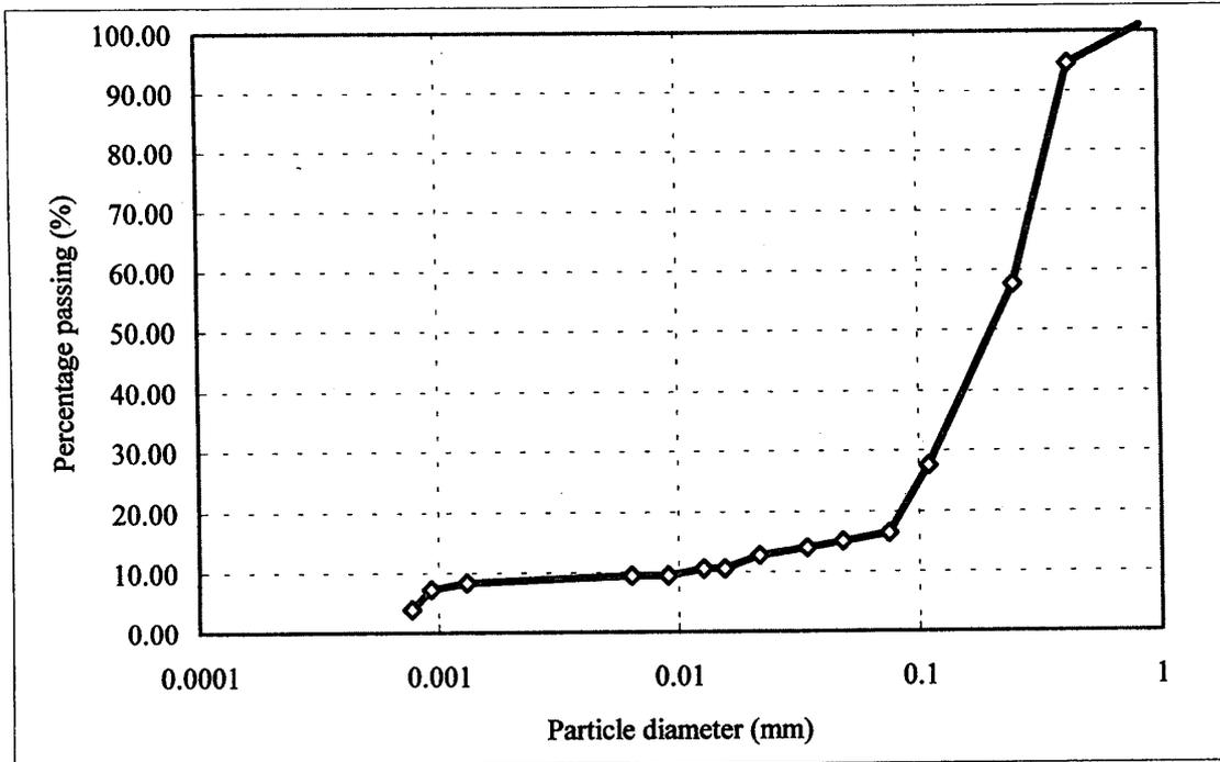
Fig. 1 Particle size distribution curve of the soil used in pullout test
