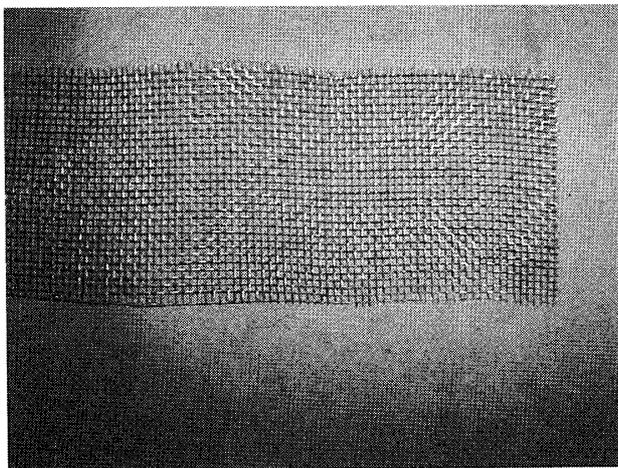
**Fig. 4c** Small grid steel wire mesh (Type III)
