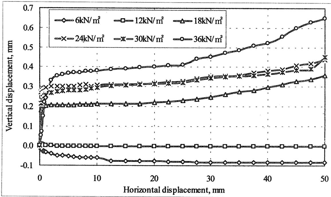
Fig. 12 Dilatancy behavior of pullout test, Type III (Woven square mesh, 3mm) reinforcement, Sandy soil with 14.36% water content.
