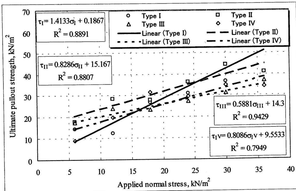
Fig. 16 Relationships between ultimate pullout strength and applied normal stress.
