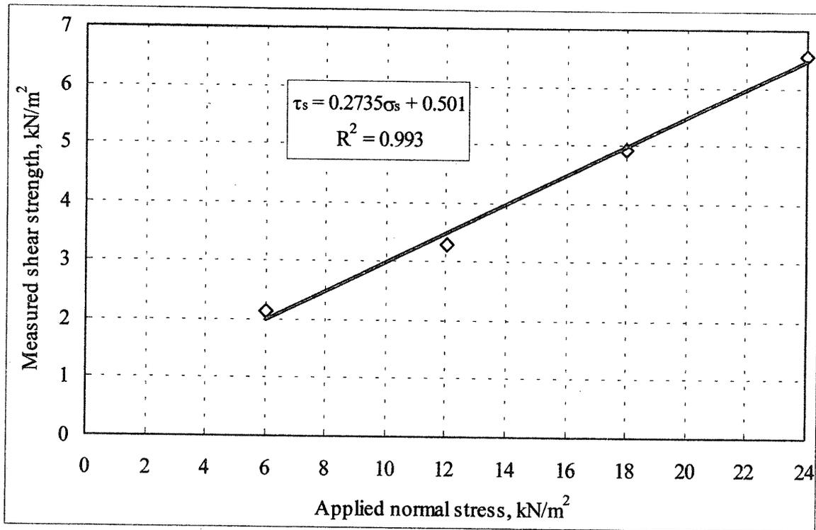
Fig. 3 Relationship of measured shear strength and applied normal stress for soil
