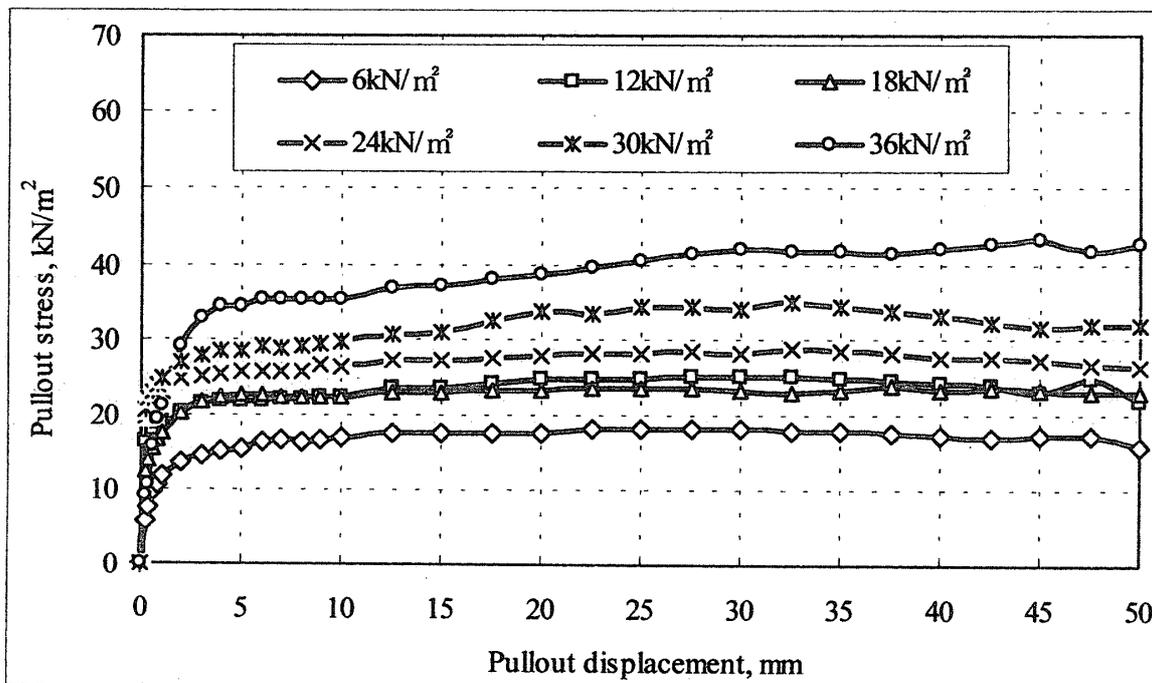
Fig. 8 Pullout stress-displacement curve, Type III (Woven square mesh, 3mm) reinforcement, Sandy soil with 14.36% water content.
