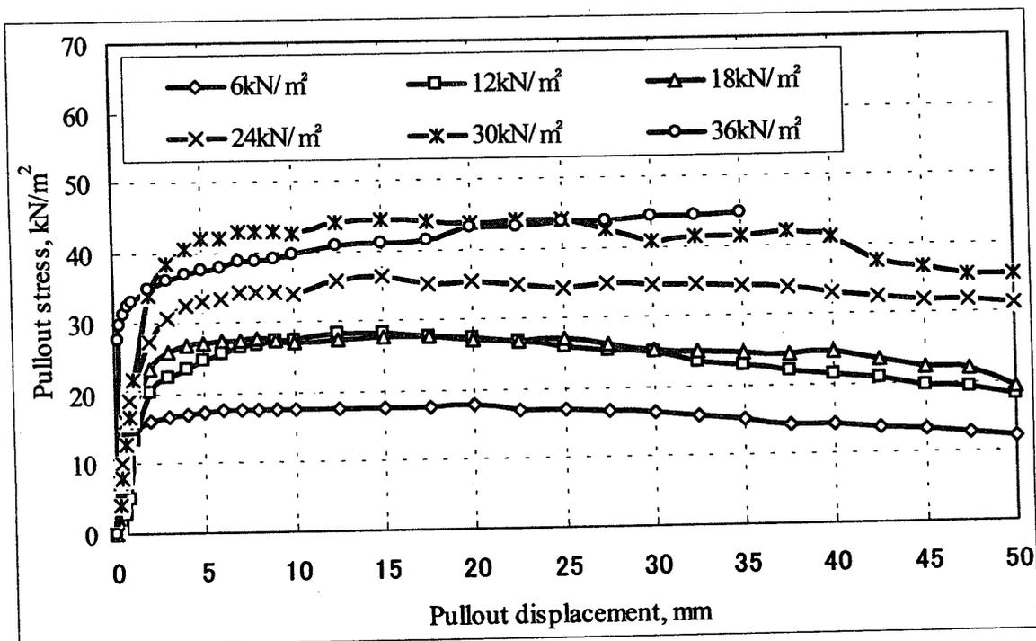
Fig. 7 Pullout stress-displacement curve, Type II (Nylon) reinforcement, Sandy soil with 14.29% water content.
