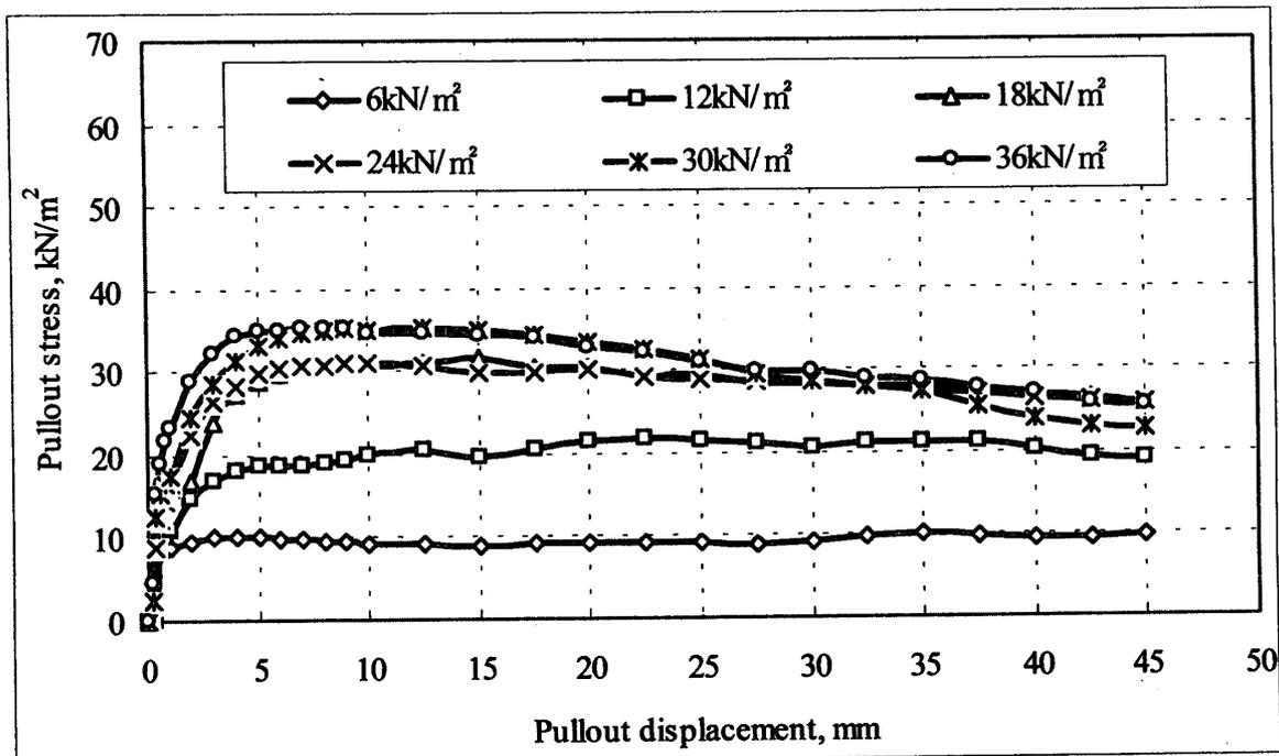
Fig. 9 Pullout stress-displacement curve, Type IV (Woven square mesh, 14mm) reinforcement, Sandy soil with 14.56% water content.
