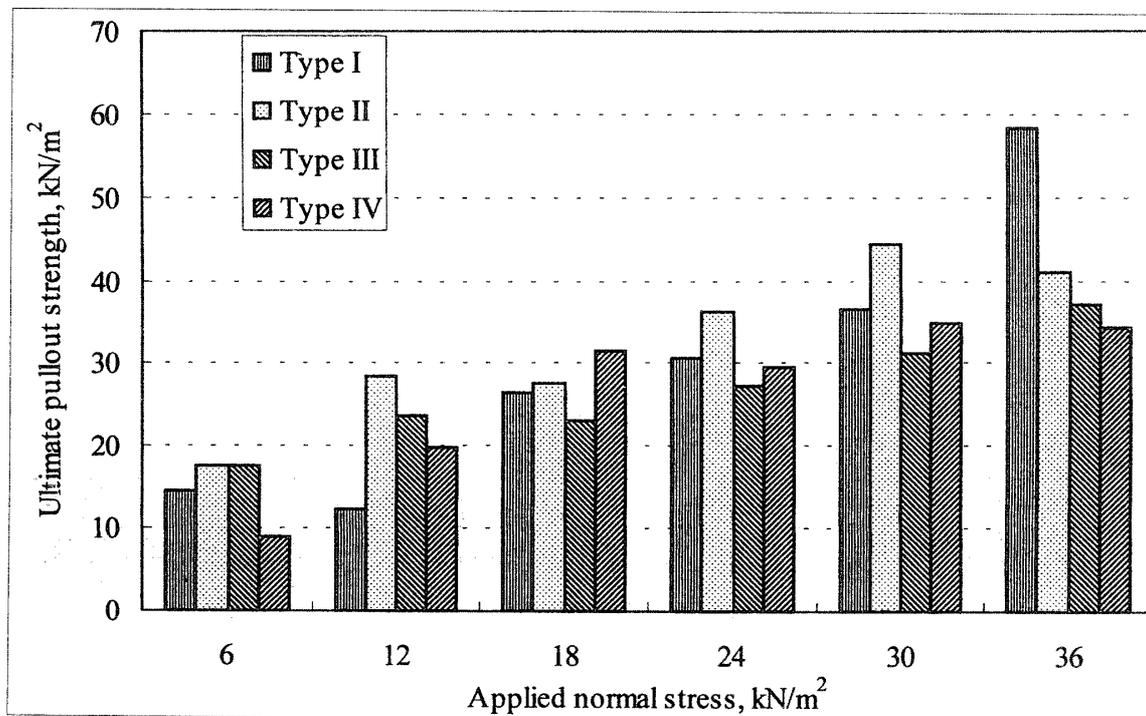
Fig. 15 Comparison of ultimate pullout stresses for geosynthetic and wire mesh under various applied normal stress conditions.
