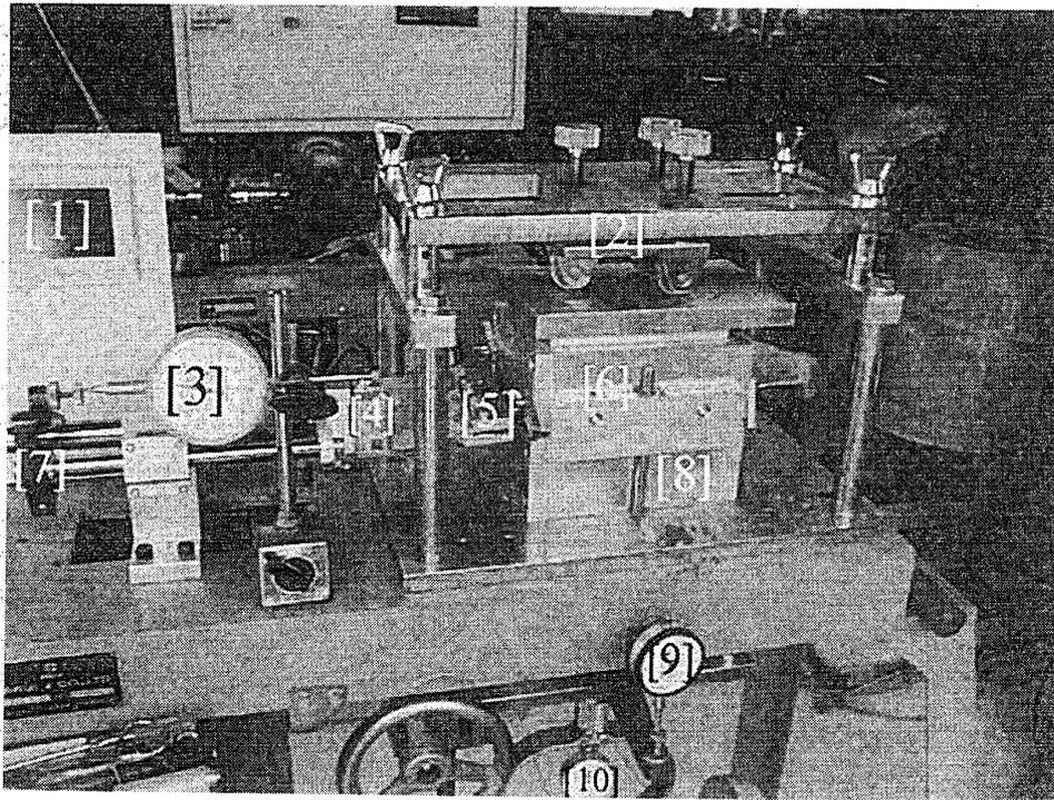
Fig. 5 Pullout and shear test apparatus of Soil-geosynthetics interaction
