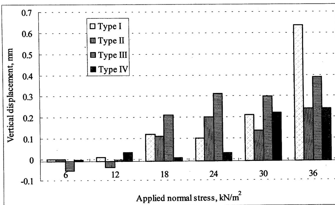
Fig. 14 Comparison of volumetric changes of pullout tests with four types of reinforcements
