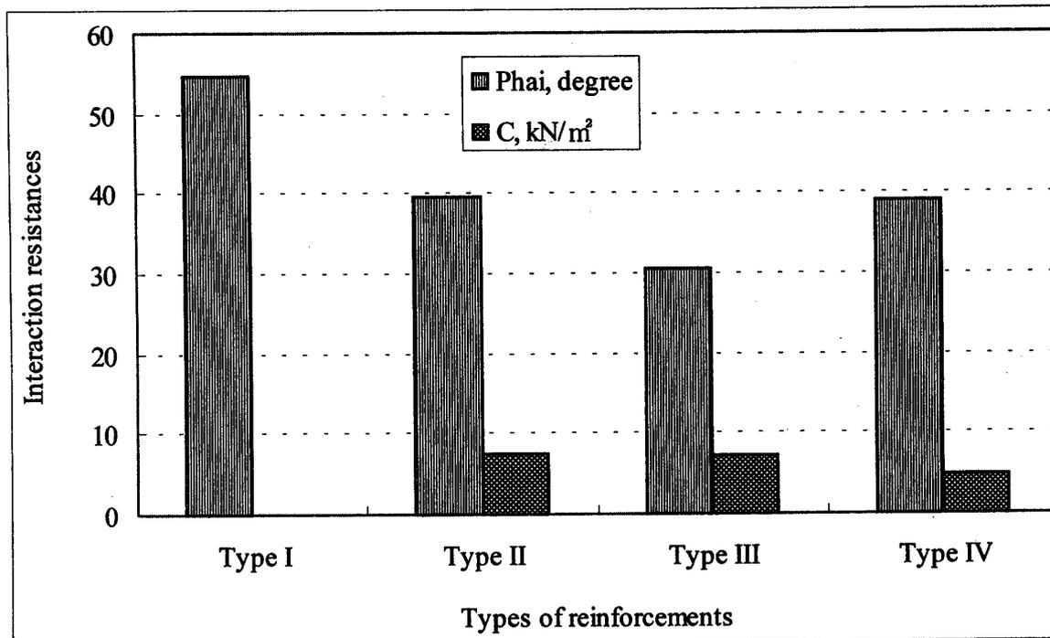
Fig. 17 Relationships between interaction resistances and reinforcement types.
