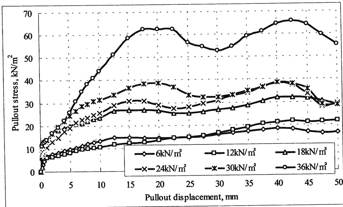
Fig 6 Pullout stress-displacement curve, Type I (Fortrac) reinforcement, Sandy soil with 14.63% water content.
