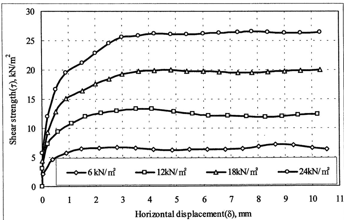
Fig. 2 Relationships of shear strength and horizontal displacement for soil
