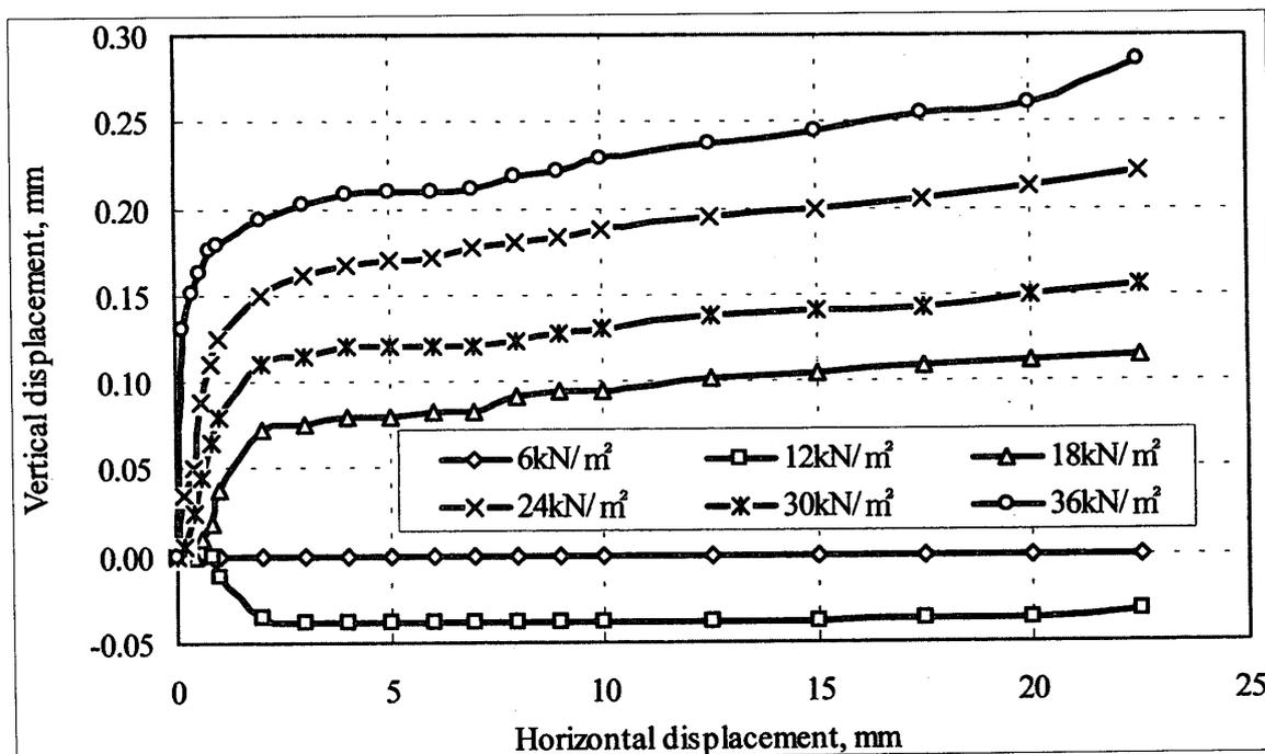
Fig. 11 Dilatancy behavior of pullout test, Type II (Nylon, 2mm) reinforcement, Sandy soil with 14.29% water content.
