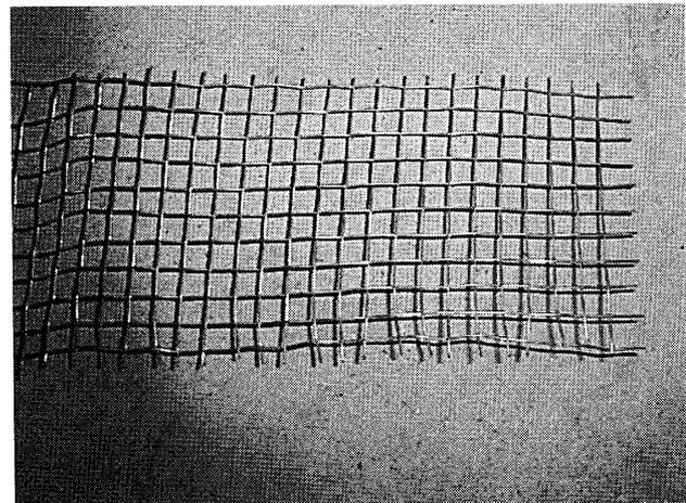
**Fig. 4d** Large grid steel wire mesh (Type IV)**Fig. 4** Physical appearance of geosynthetics and woven square wire meshes
