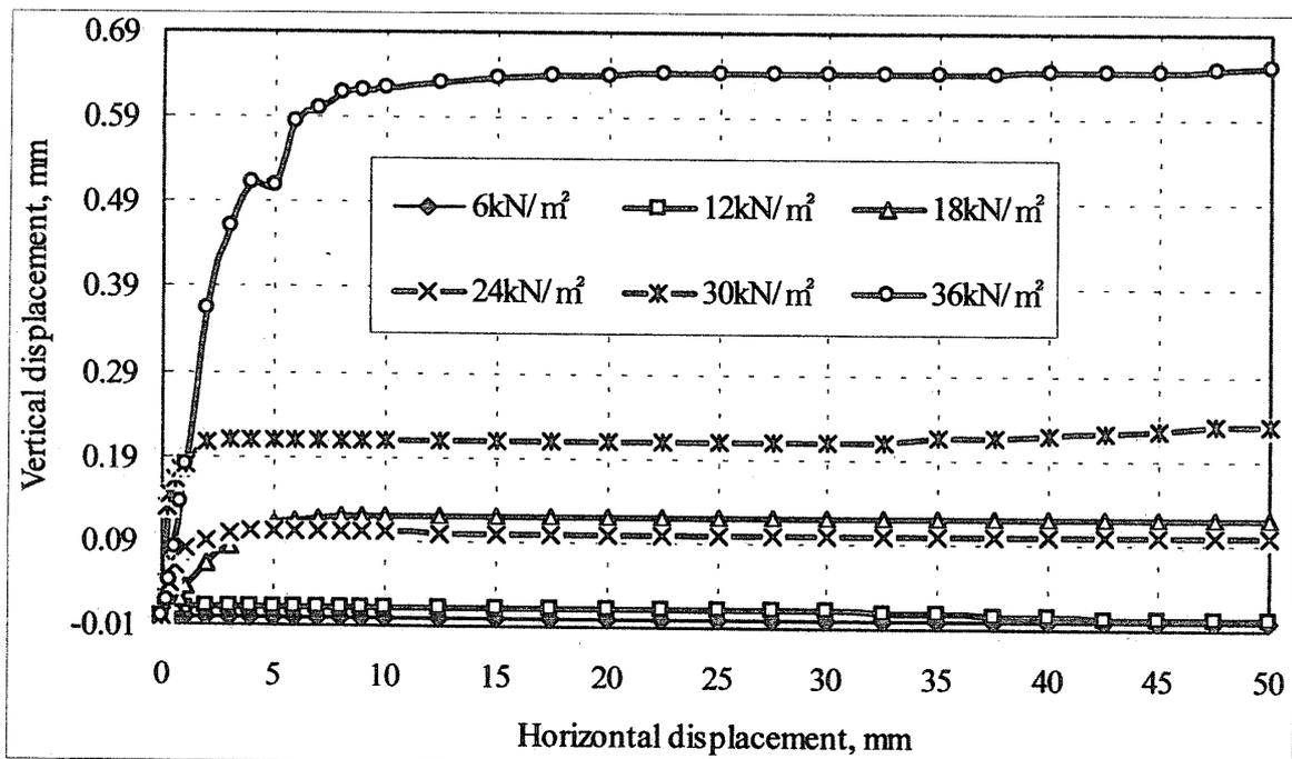
Fig. 10 Dilatancy behavior of pullout test, Type I (Fortrac) reinforcement, Sandy soil with 14.63% water content.
