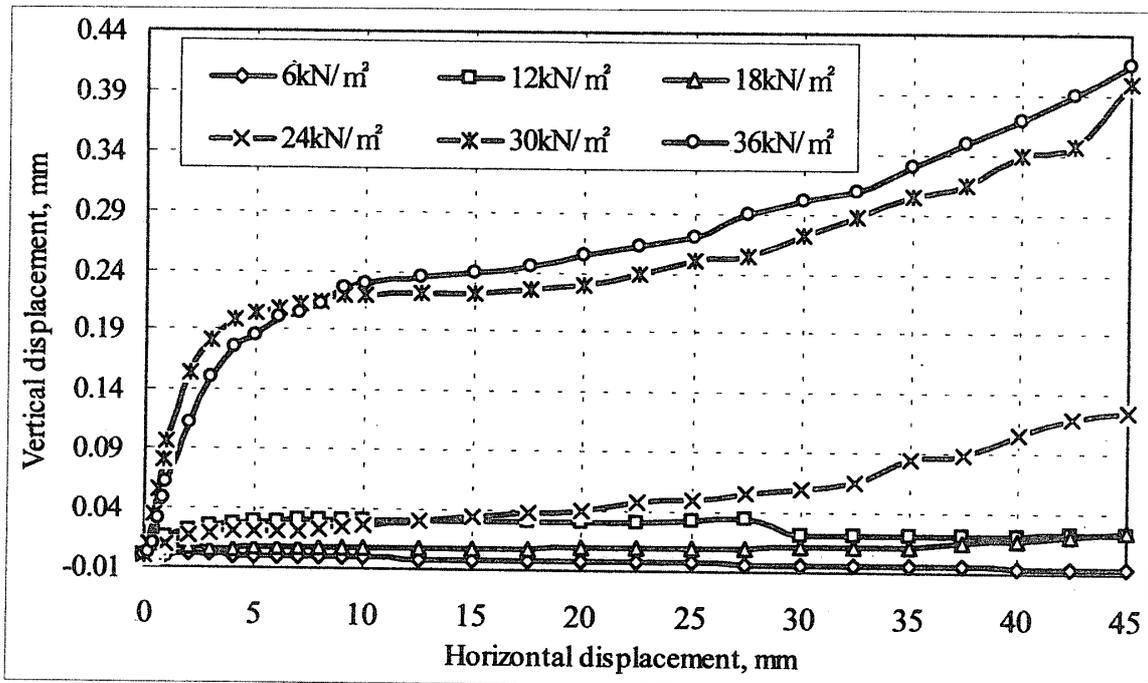
Fig. 13 Dilatancy behavior of pullout test, Type IV (Woven square mesh, 14mm) reinforcement, Sandy soil with 14.56% water content.
