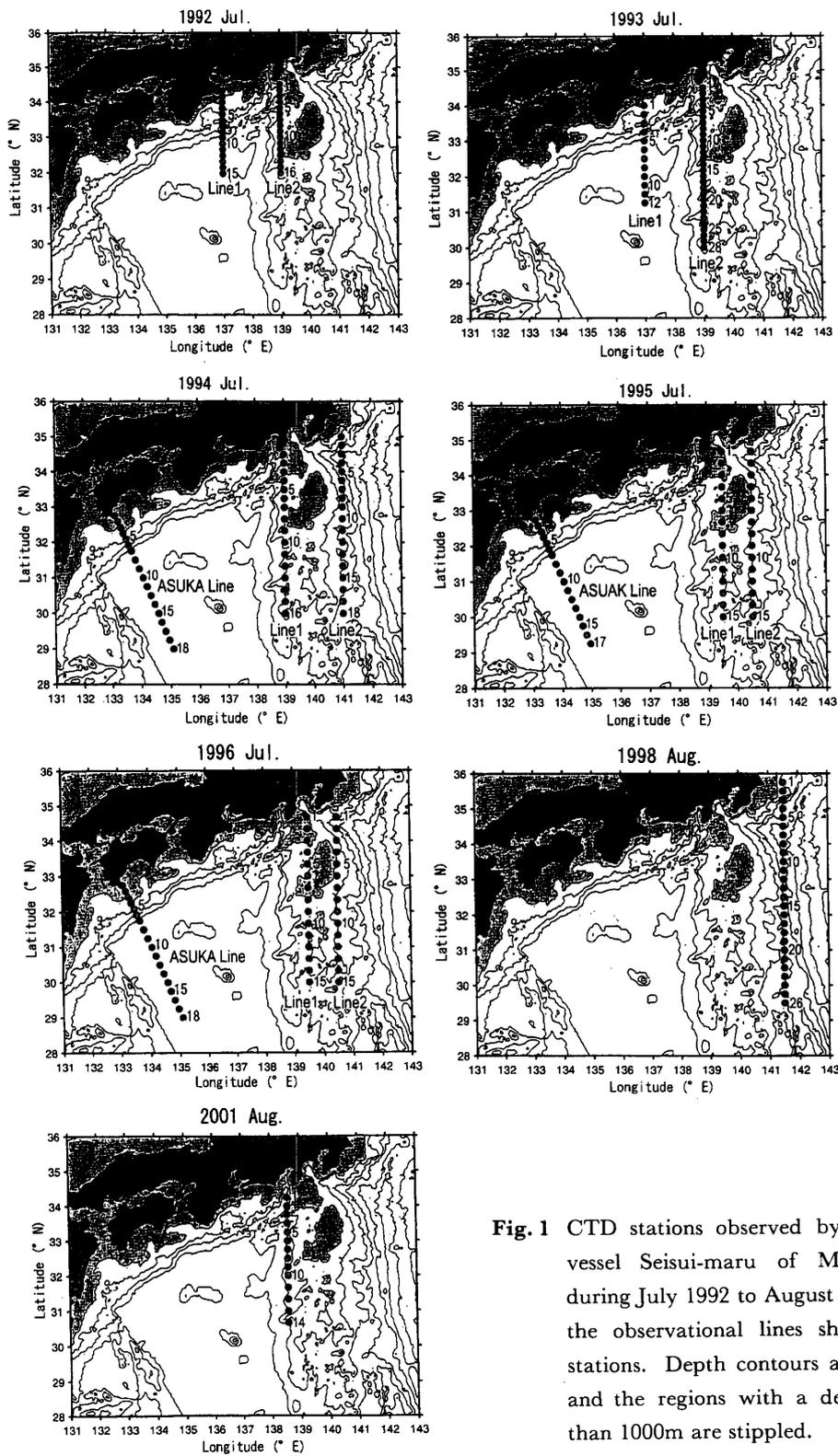
**Fig. 1** CTD stations observed by the training vessel Seisui-maru of Mie University during July 1992 to August 2001. Dots in the observational lines show the CTD stations. Depth contours are also shown and the regions with a depth shallower than 1000m are stippled.
