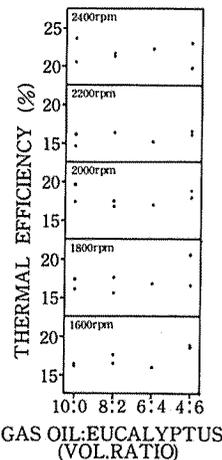
Fig. 14. — Relationships between blend ratio and thermal efficiency
