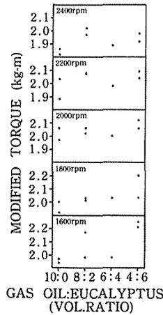
Fig. 6. — Relationships between blend ratio and modified torque
