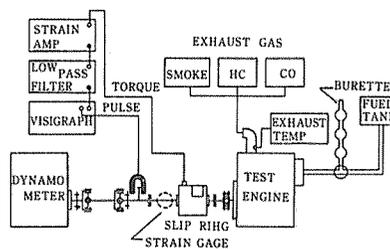
Fig. 2. Diagram of experiment apparatus
