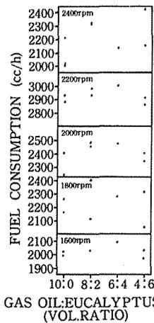
Fig. 8. — Relationships between blend ratio and fuel consumption
