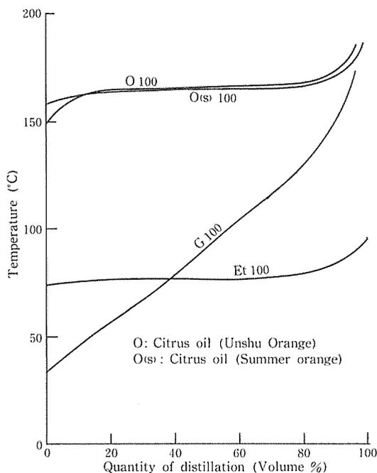
Fig. 2-1. Distillation curve.
