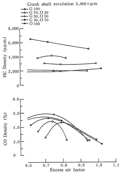
Fig. 4-2. Analysis of exhaust gas.
