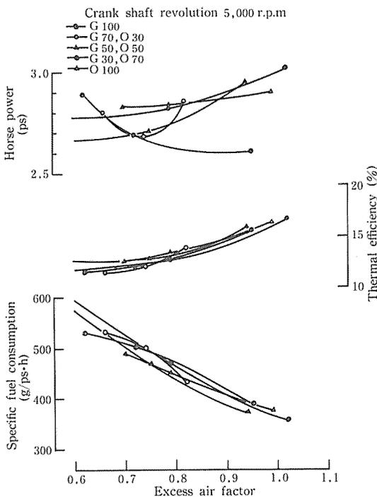
Fig. 4-1. Engine performance test.
