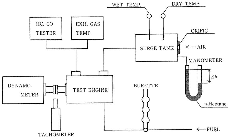
Fig. 3. DIAGRAM OF EXPERIMENTAL APPARATUS.
