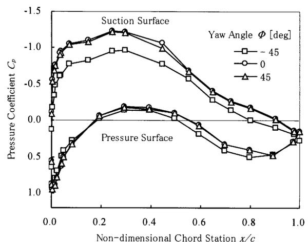
Fig. 11 Pressure distribution at  $\alpha = 10$  degrees in several yawed conditions
