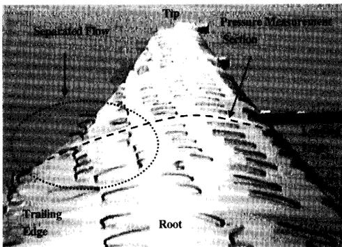
Fig. 13 Flow visualization on suction surface at  $\Psi = 0$  degree ( $\alpha = 10.6$  degrees,  $\beta = 9.5$  degrees,  $\Phi = -49.1$  degrees and  $Re = 3.5 \times 10^5$ )
