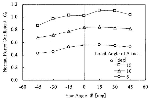
Fig. 8 Normal force coefficient  $C_n$  against yaw angle  $\Phi$
