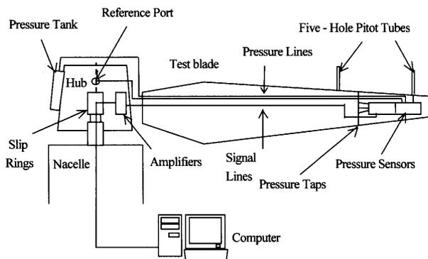
Fig. 4 Measurement system
