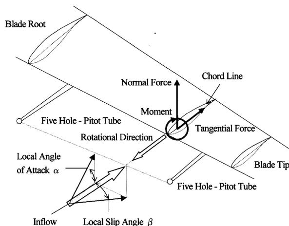
Fig. 5 Definition of normal force, tangential force, moment, local angle of attack and local slip angle
