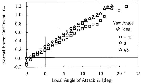
(a) Normal force coefficient  $C_n$  against local angle of attack  $\alpha$
