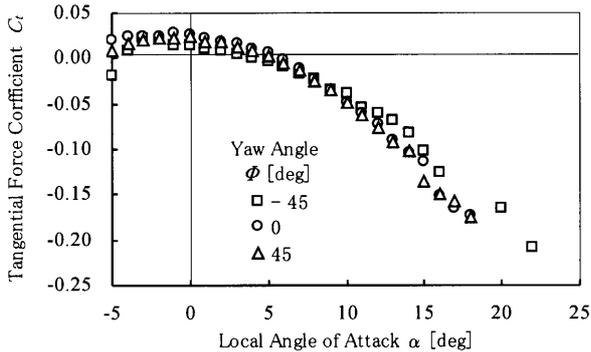
(b) Tangential force coefficient  $C_t$  against local angle of attack  $\alpha$
