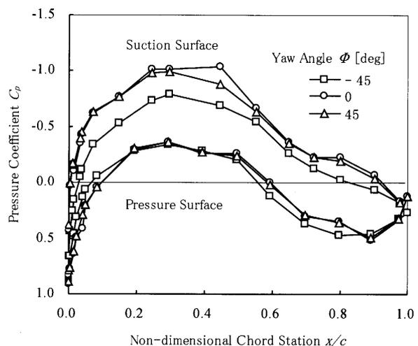
Fig. 12 Pressure distribution at  $\alpha = 5.5$  degrees at  $\psi = 270$  degrees in several yawed conditions
