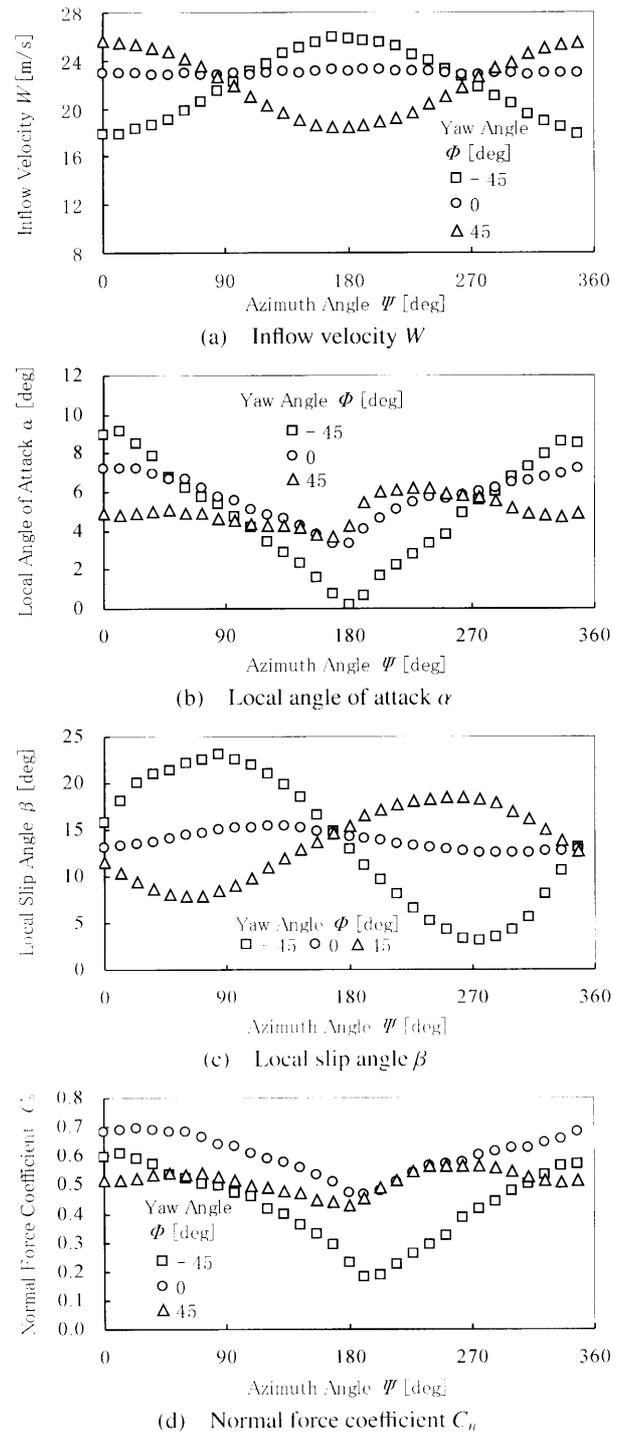
Fig. 10 Change of section characteristics due to azimuth angle  $\Psi$  in several yawed conditions
