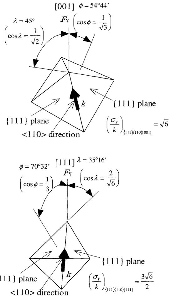
Fig. 4 Equally stressed systems upon pulling along  $[001]$  and  $[111]$ <sup>(9)</sup>
