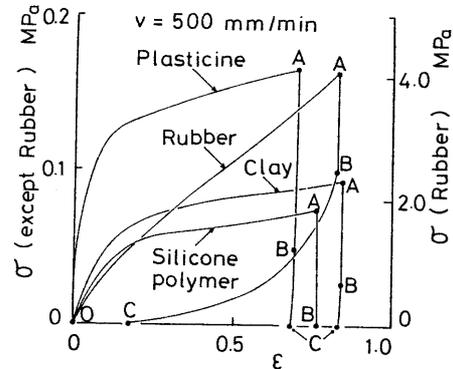
Fig. 3 Compressive stress-compressive strain ( $\sigma - \epsilon$ ) curves in the low speed compression test.
