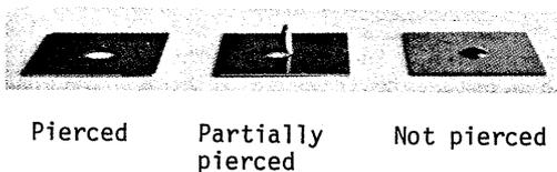
Fig. 9 Samples obtained in the piercing test.
