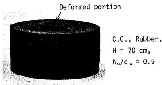
Fig. 11 Appearance of the rubber specimen after piercing.
