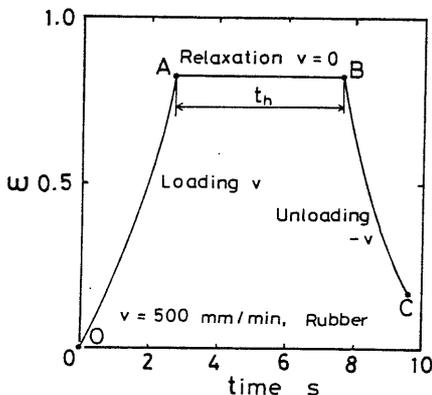
Fig. 2 Strain path in the low speed compression test.
