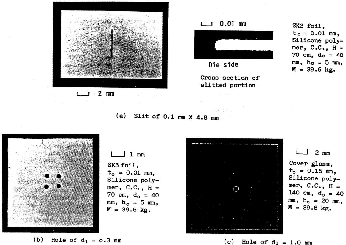
Fig. 12 Piercing of small holes and glass sheet.
