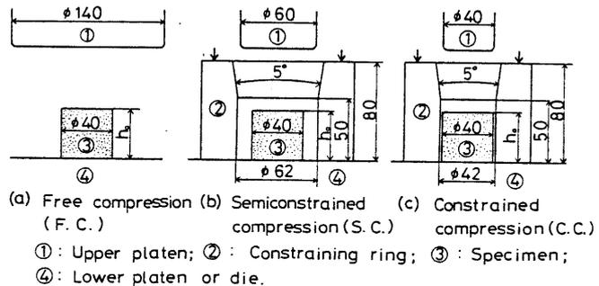
Fig. 4 Schematic drawing of compression methods.
