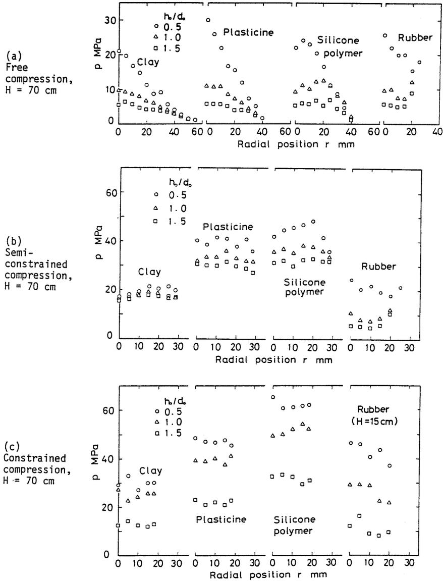
Fig. 8 Radial distribution of pressures in the flat-platen compression test.
