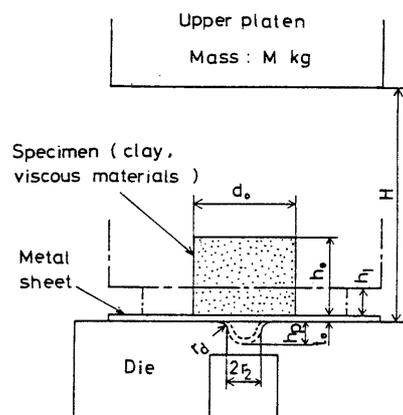
Fig. 1 Schematic drawing of stretch-forming by impulsive free compression of a viscous material.
