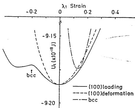
Fig. 2. Variations of the crystal energy with strain.
