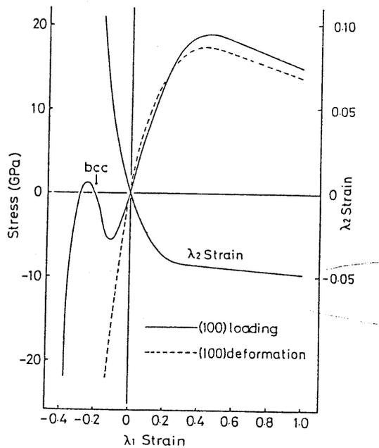
Fig.4. Stress-strain curves.
