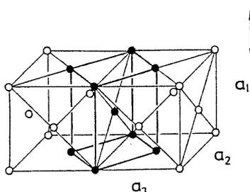
Fig. 1. The relation of the face centered cubic to the body centered tetragonal (in the case of  $c$ -axis parallel to the loading axis  $a_1$ ).
