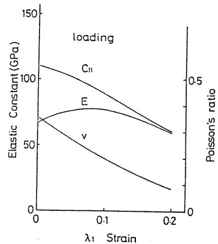
Fig.5. Variations of the elastic constants with strain in the loading mode.
