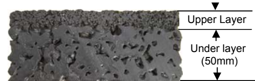
Fig.2 A double layered POC sample Upper layer = 4, 8 & 12mm thick
