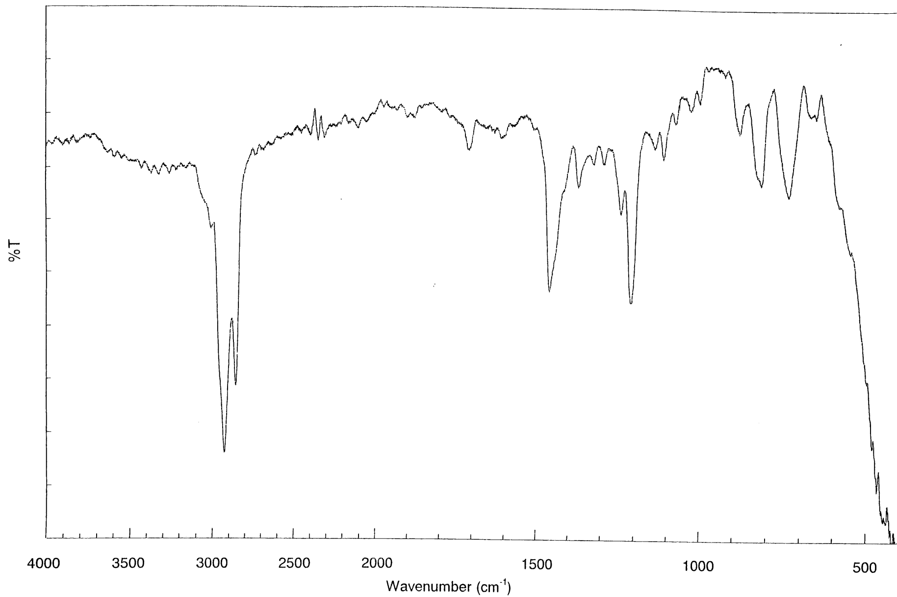
Figure 6. IR spectrum of 2,7-bis (bromomethyl) -9,9'-dioctylfluorene ( 3 ) (NaCl)
