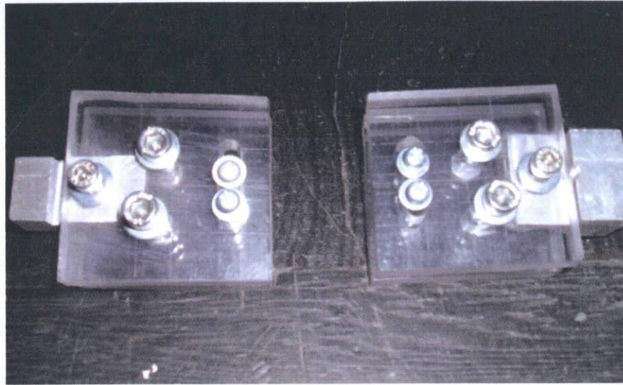
Fig.3-8 Jig for tensile exam.
