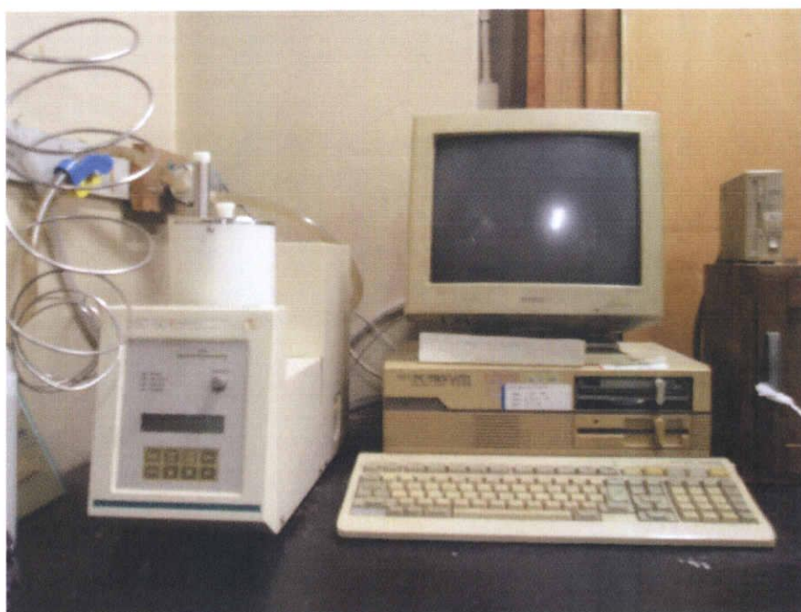
Fig.3-7 DSC measurement system
