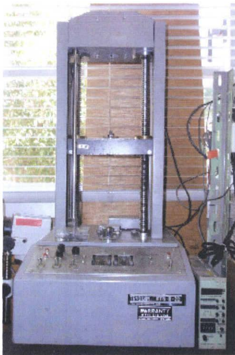
Fig.3-9 Tensile testing machine
