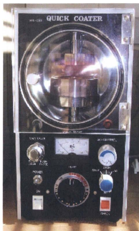
Fig.3-14 Plate coating machine
