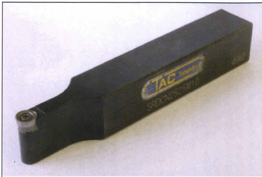
Fig.3.11 Photograph of Normal cutting tool (Circular chip , \phi 10)
