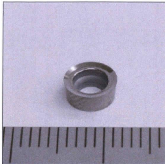
Fig.3.10 Photograph of chip used (Circular chip , \phi 6)
