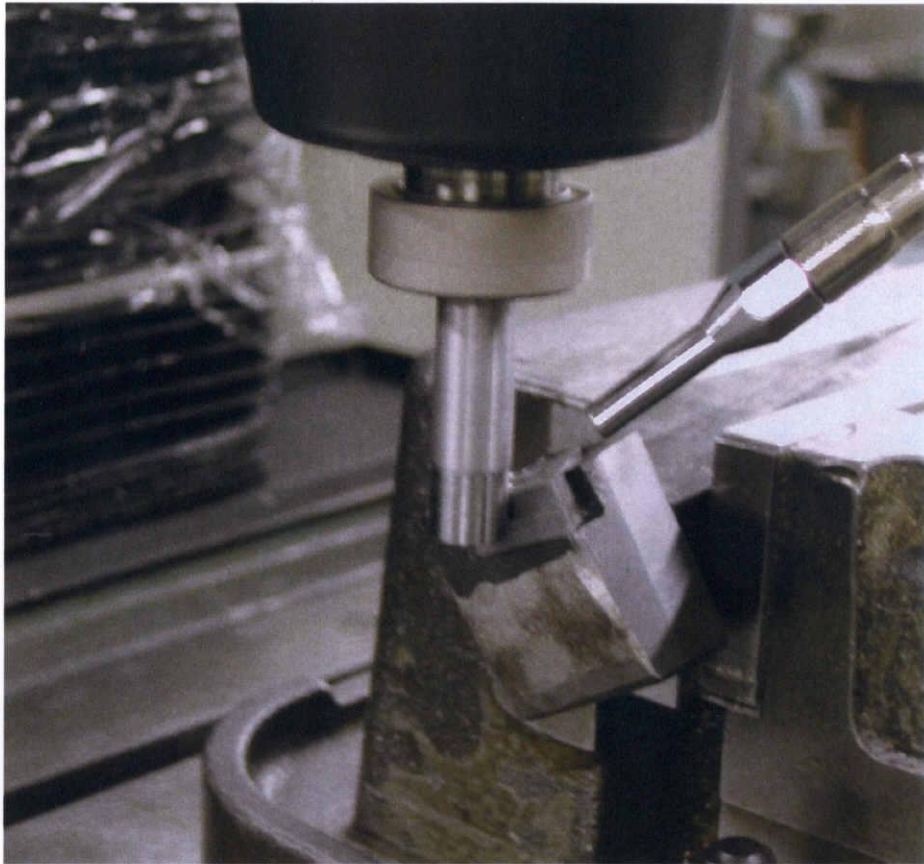
Fig.3.2 Setup for external cylindrical cutting
