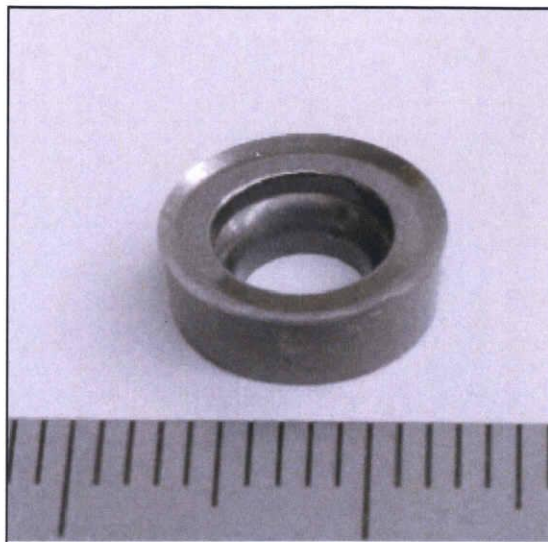
Fig.3.9 Photograph of chip used (Circular chip , \phi 10)
