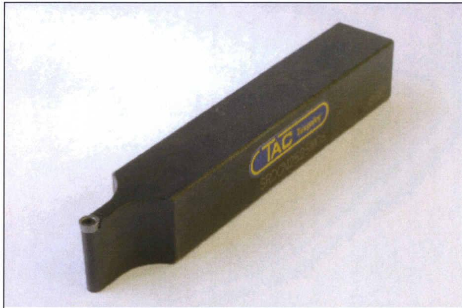
Fig.3.12 Photograph of Normal cutting tool (Circular chip , \phi 6)
