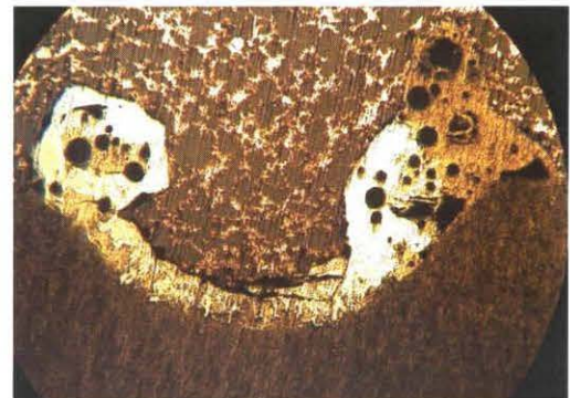
Fig.5-17 Cross-section of wire and base metal
