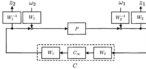
(b) Equivalent closed loop system.
