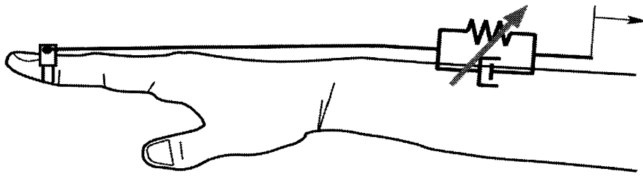
Fig.2.8 Model of an assist system of the finger by using impedance control
