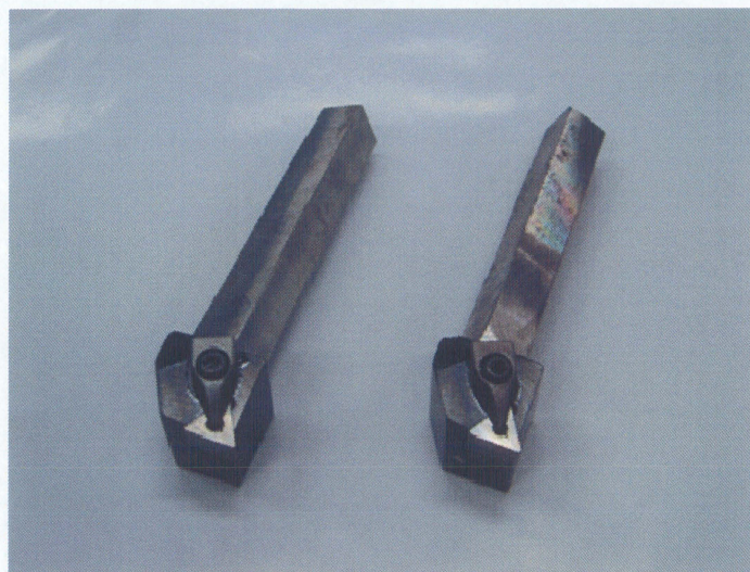
Fig.4.2 Photograph of oblique cutting tools
