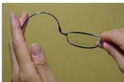
Fig.2-1 Application for glasses of frame of shape memory alloy 12)
