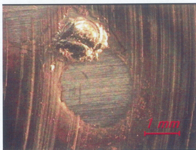
Fig.3.9 The test piece surface with sparking
