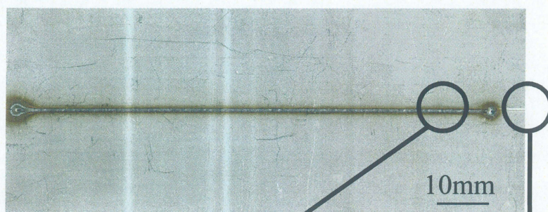
(a) Appearance of laser butt welded specimen
