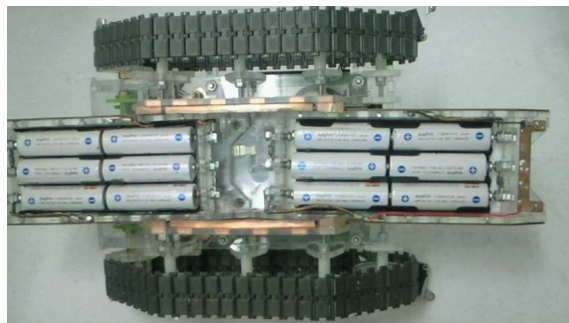
Fig. 3.15 Battery exchange mechanism
