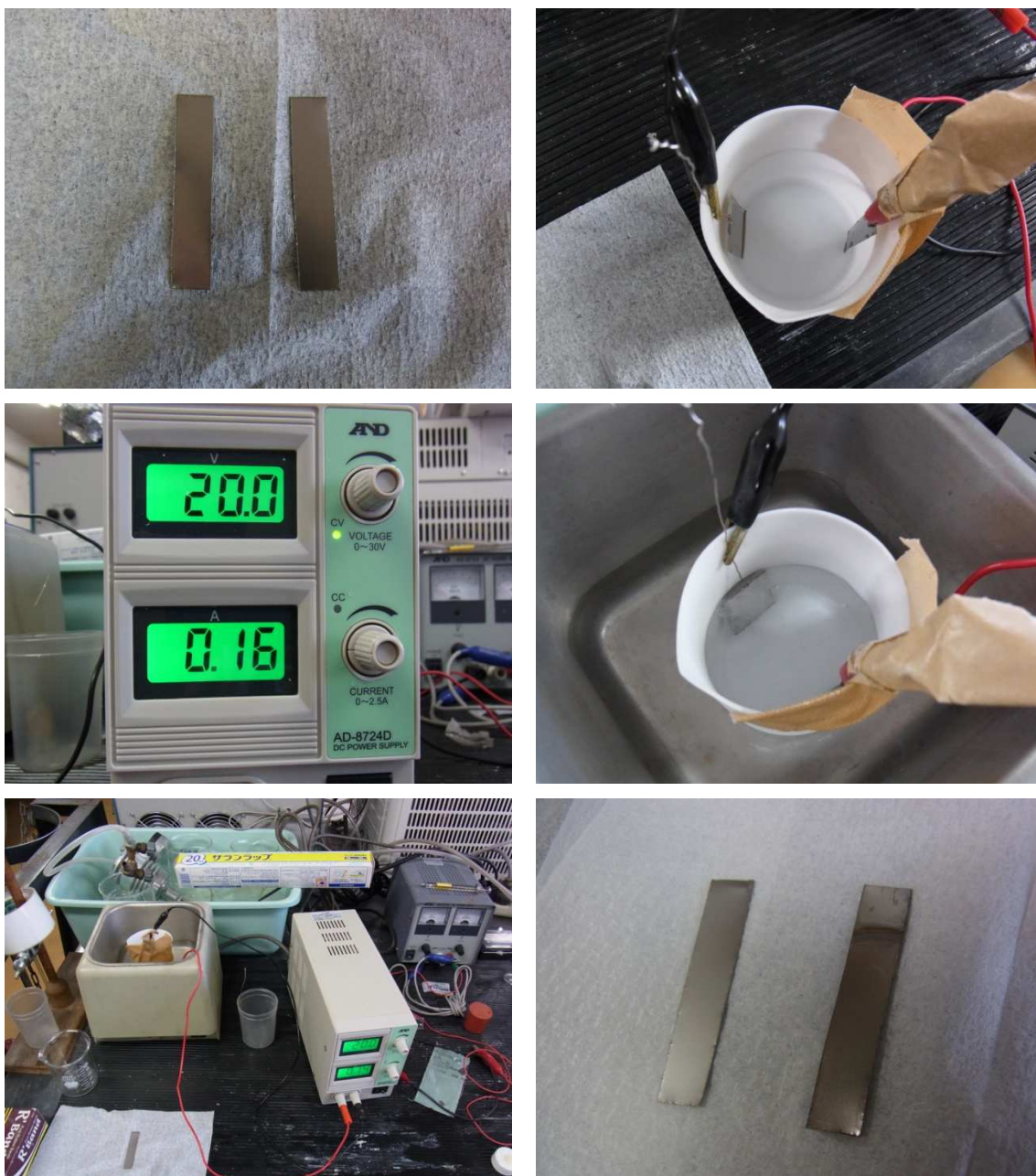
Fig. 2-3-d. Anodization reactor for TiO 2 nanotube.
