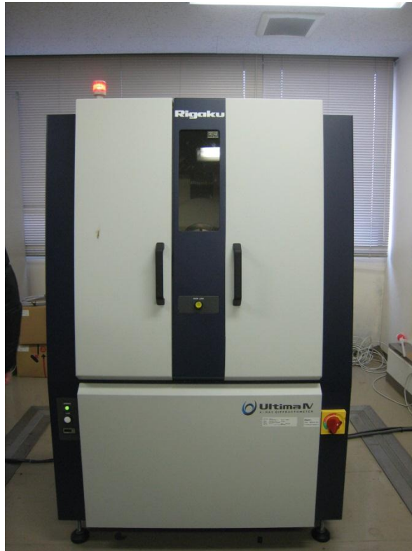
Fig.4.5 (a) Powder X-ray diffractometer (Ultima IV)
