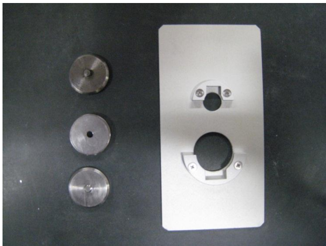
Fig.4.2 (b) Mold of making pellet
