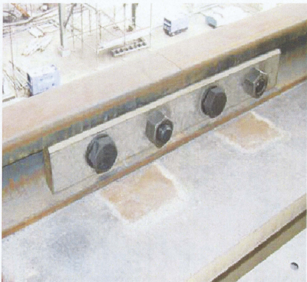
Fig.2-1-5 Locking joint material of Fe-Mn-Si shape memory alloy (15)
