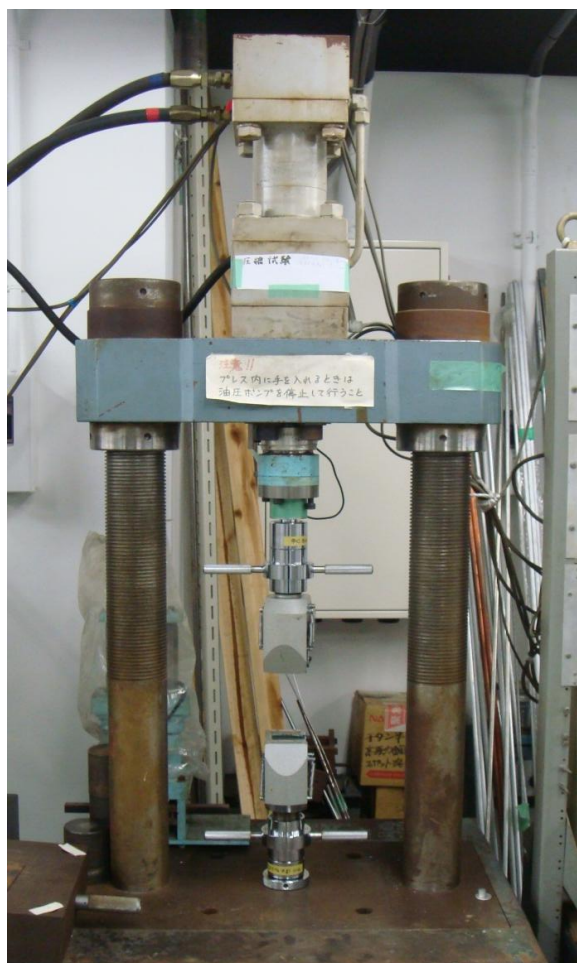
Fig.3.13 Hydraulic servo press used for tensile test
