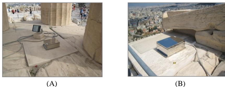
Fig. 2-9 Servo accelerographs. (A) Master sensor, and (B) Slave sensor
