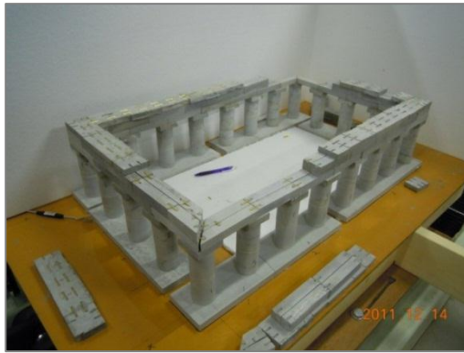
Fig. 4-6 Horizontal clamps between beams
