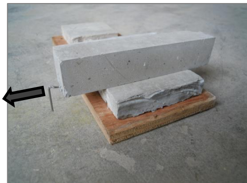
Fig. 4-9 Friction coefficient test
