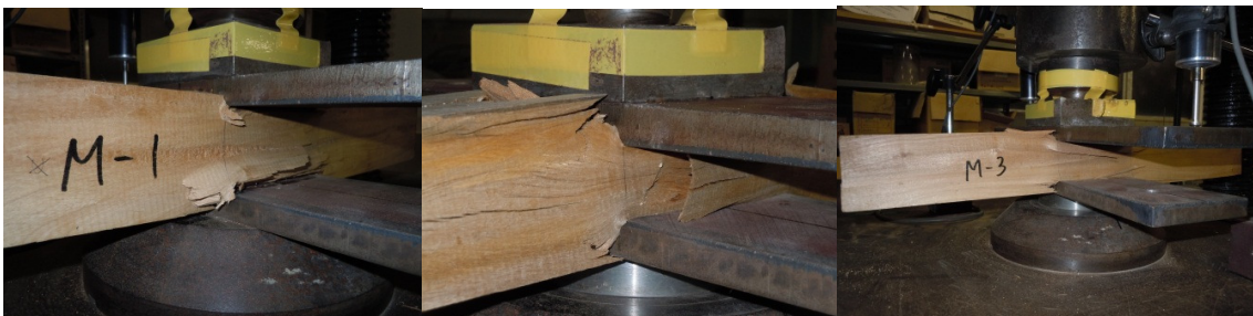
Photo.5-9 Failure mode of Manawadono (from the left: M-1, M-2, M-3)
