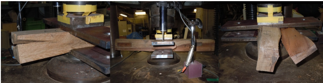
Photo.5-8 Failure mode of Afoa (from the left: A-1, A-2, A-3)
