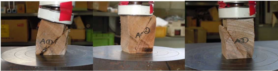
Photo.5-12 Failure mode of Afoa (from the left: A1, A2, A3)
