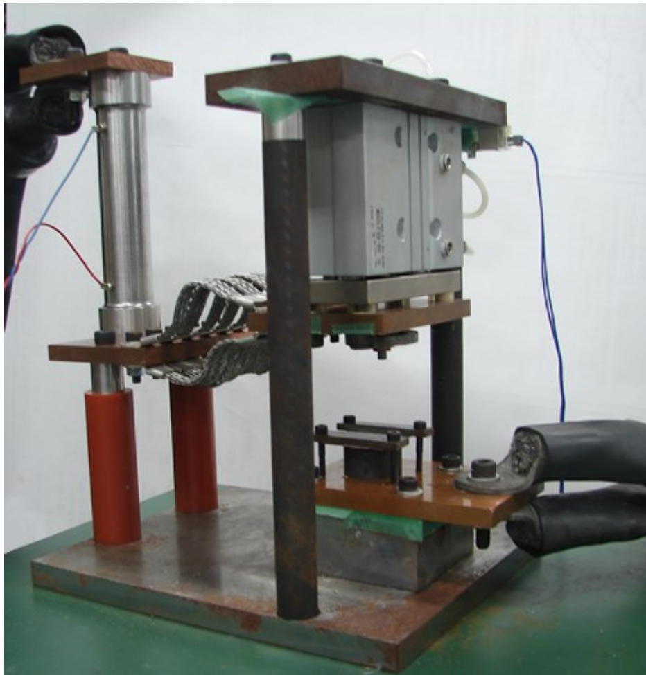
Fig.3.2 Equipment of the local hardening method using resistance heating
