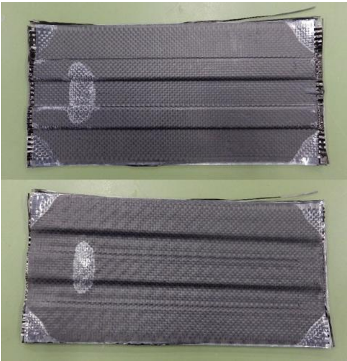
Fig.4.8 C-FRP molded by using mold which is showed Fig.4.7
