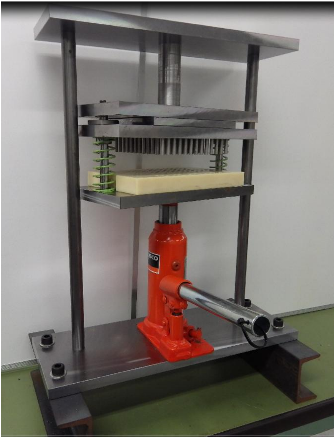
Fig.2.15 Device for punching holes on polyethylene resin sheets
