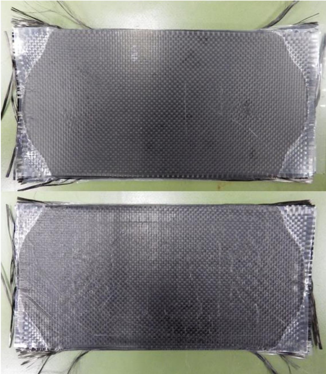
Fig.4.6 C-FRP molded by stopping for two minutes in a test piece both ends and moving one minute to the opposite direction
