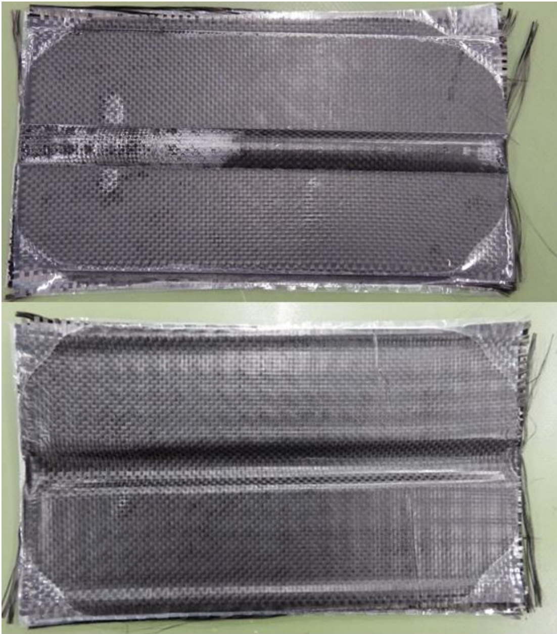
Fig.4.10 C-FRP molded by using mold which is showed Fig.4.9
