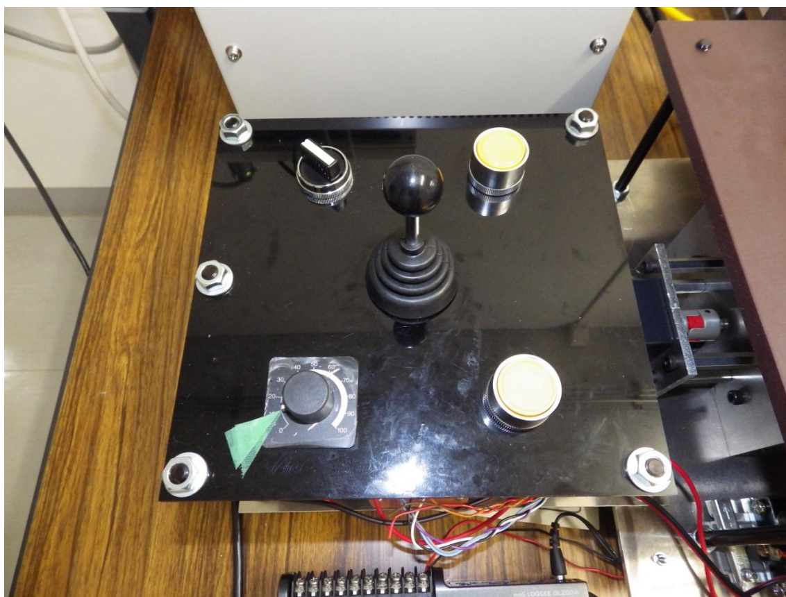
Fig.2.11 Controller to operate a coil
