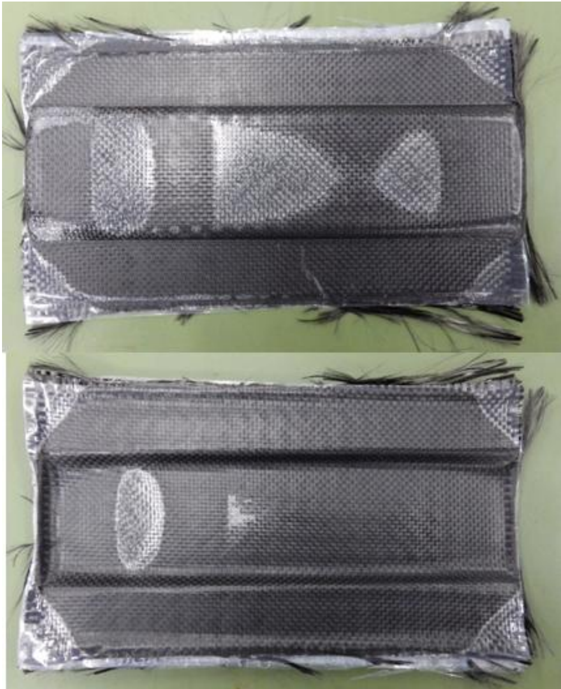
Fig.4.11 C-FRP molded by using mold which has wide width groove
