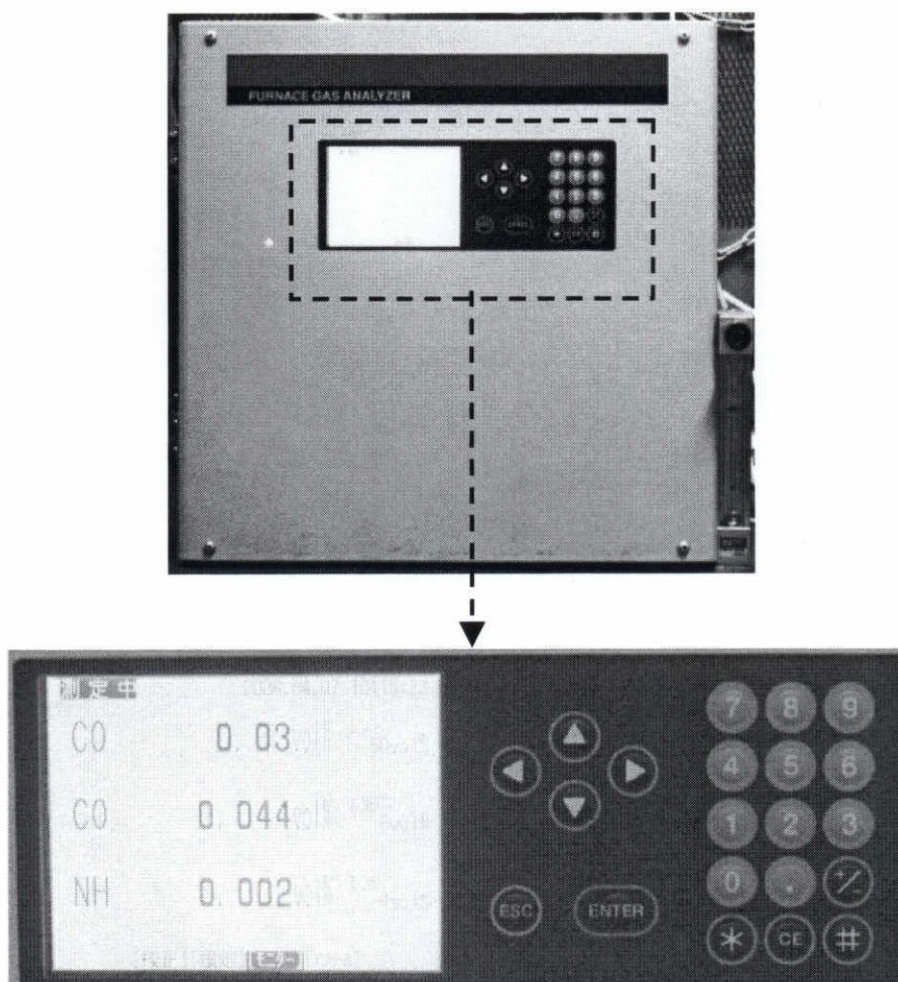
Fig. 4-5 Non Dispersive Infrared Red analyzer (NDIR).
