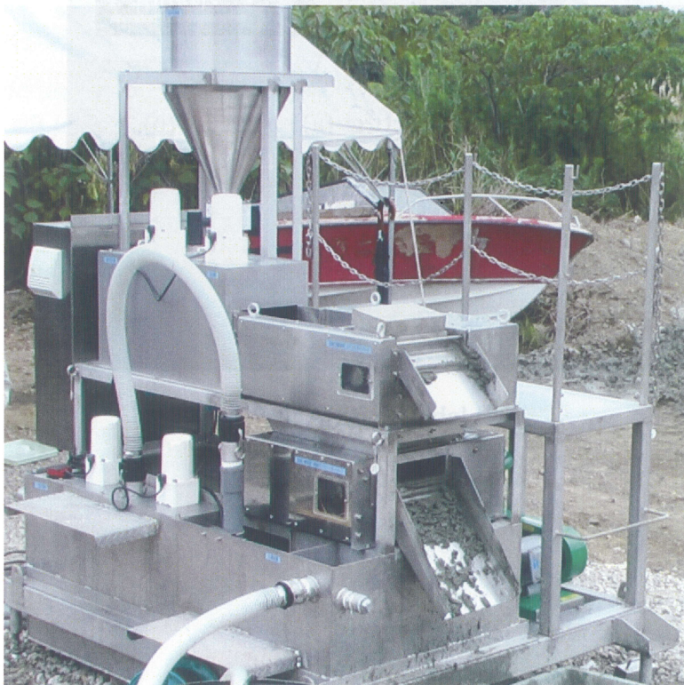
Figure 2-2: Solidification method “Hi-Biah-System” of sediments.
