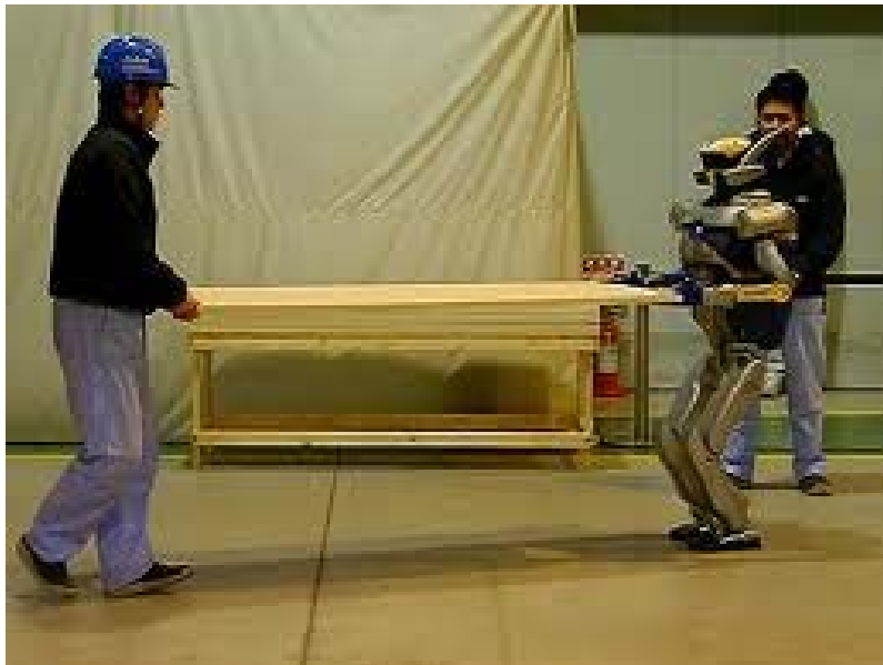
Fig. 3 HRP-2 carrying a panel with a human (Yaskawa Electric, Shimizu Corporation, Kawada Industries, AIST)[2]. Example of Synchronous, Collocated, Side by Side human robot cooperative motion.
