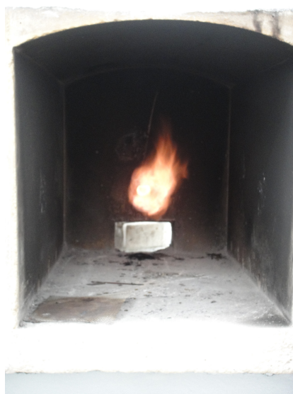
Fig. 4-10 Ignition of biomass producer gas at the primary burner
