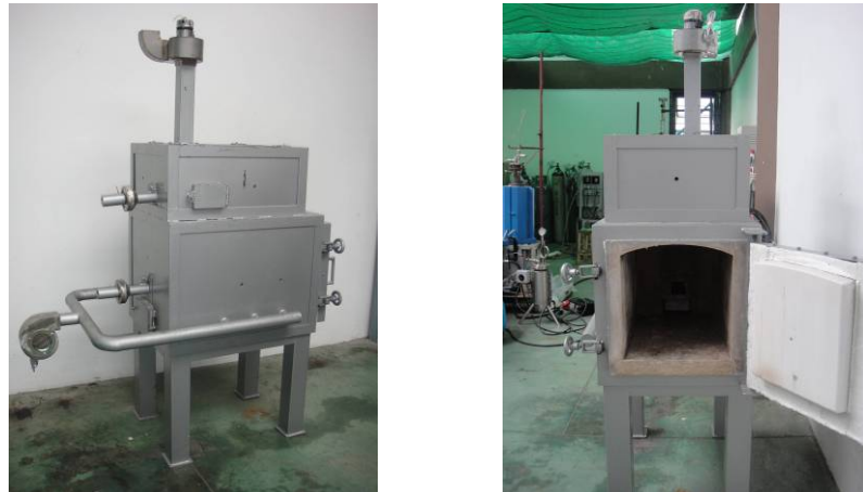
Fig.4-6 Prototype of high-moisture material's double-chambered incinerator
