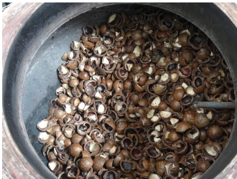
Fig. 4-9 Introduction of biomass fuel into the gasifier
