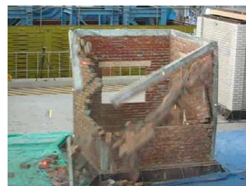
6. Collapse of two walls with two ring beams
