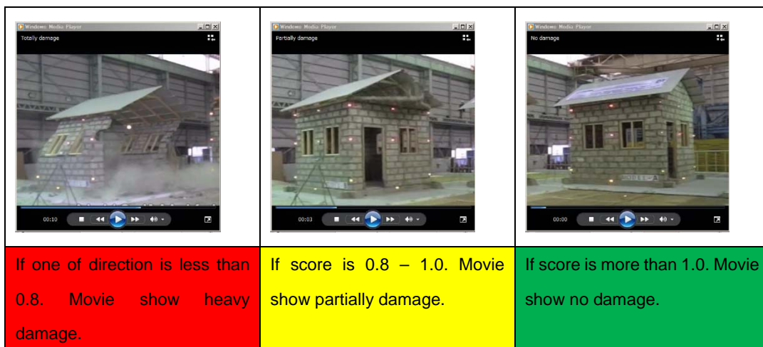
(B) According to score, movie of damage is pop-up
