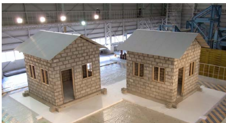
Fig.63 Model structure on the shaking table
