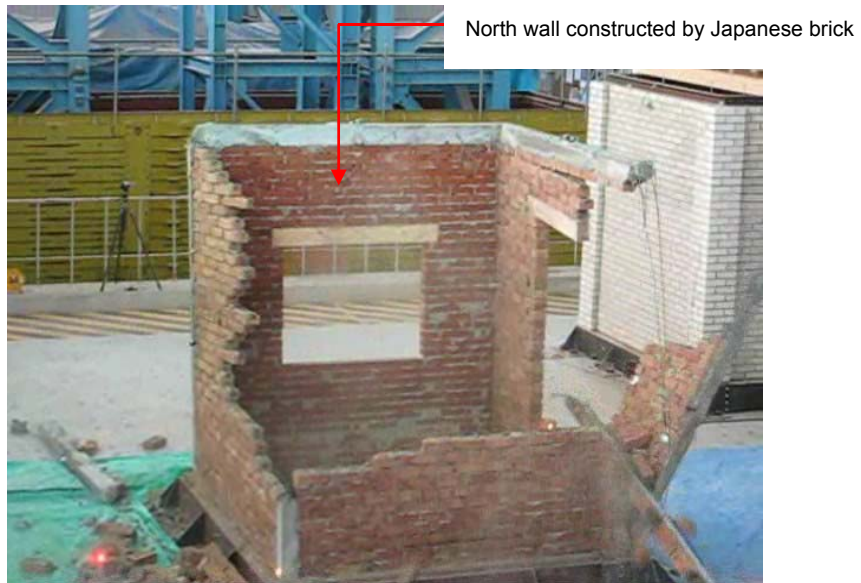
Fig.62 North wall did not collapsed in this test
