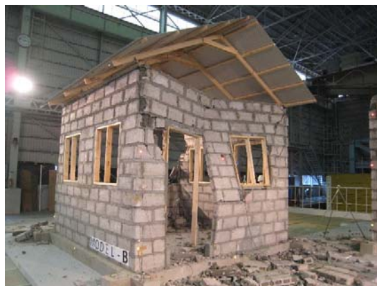
Fig. 77 Out-of-Plane failure on Model B before totally collapse
