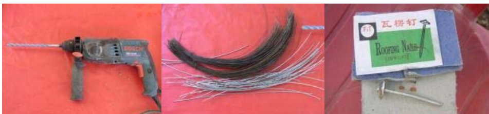
(B) Fixing tools and Materials: Drill, Bending wire, Nail for temporary fixing.
