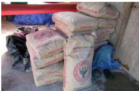
(C) For Plastering: Mortal Ratio is cement 1 : sand 4 by volume
