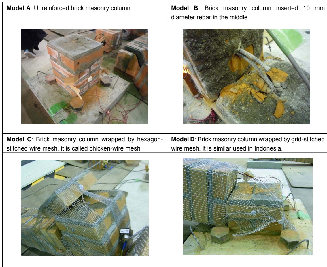
Fig.96 Condition of each model after test
