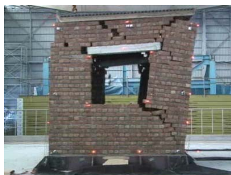
Fig. 82 Diagonal cracks in shaking table test of South-Asian model structure in Chapter 2.2
