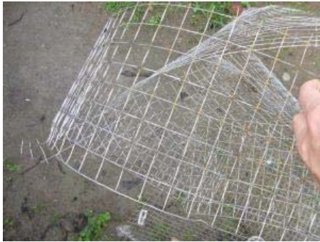
(A) Wire mesh: Galvanized Welded Wire mesh, Spacing 25 mm, 1 mm Diameter
