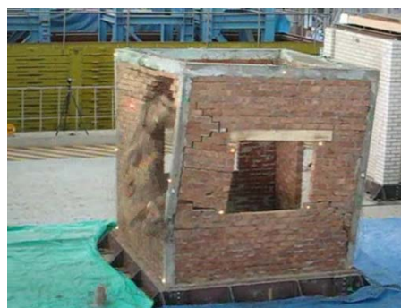
Fig. 84 Out-of-plane failure in shaking table test of South-East Asian model structure in Chapter 2.3
