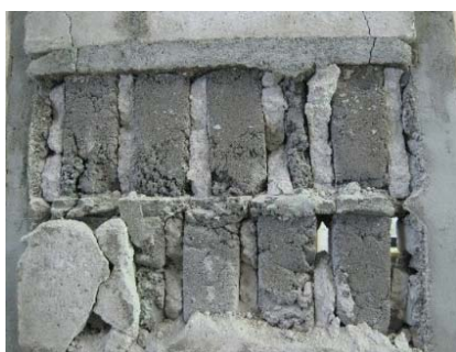
Fig.74 Face-shell of CHB fell down of Model A after shaking
